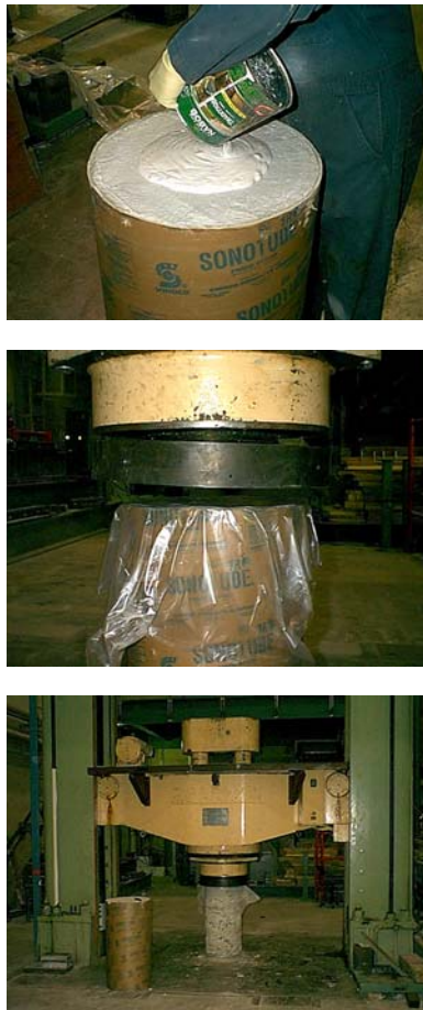
Figure 3. Top: Placing Plaster of Paris thincoat about ½-hour prior to loading. Middle: Placing loading plate on thincoat before setting. Bottom: A specimen ready to be tested.
