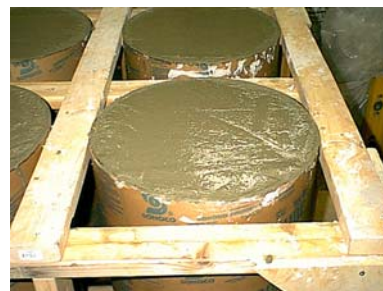
Figure 2. Top: Preparing specimens for top capping. Middle: A specimen just before top capping applied. Bottom: A specimen just after top capping applied.
