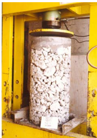
Figure 1. A typical 450 mm diameter by 900 mm high Cemented Rockfill Sample being tested for Unconfined Compressive Strength using a commercial test frame.
