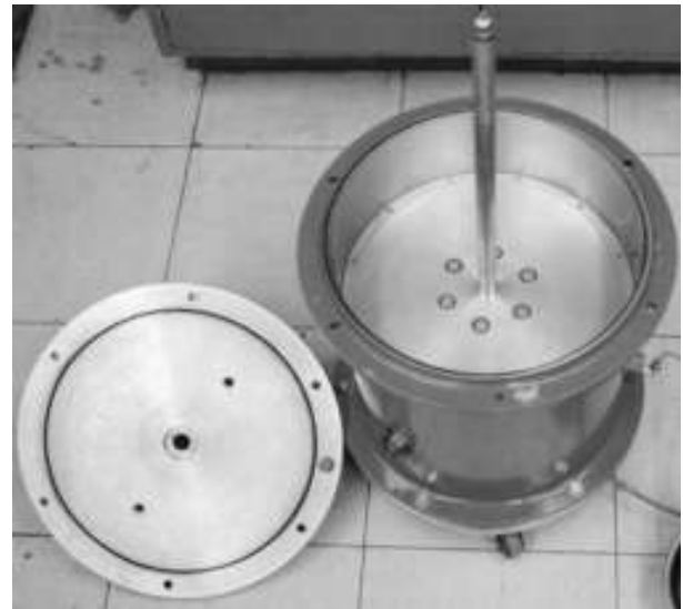
Figure 1. Large diameter slurry consolidometer, shown with upper lid removed.
