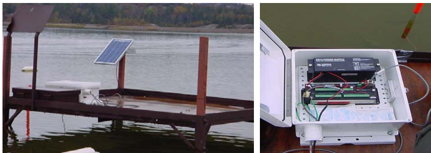
Fig 2. Photograph of the platform and data logger assembly installed at 0.75 m of water cover depth
