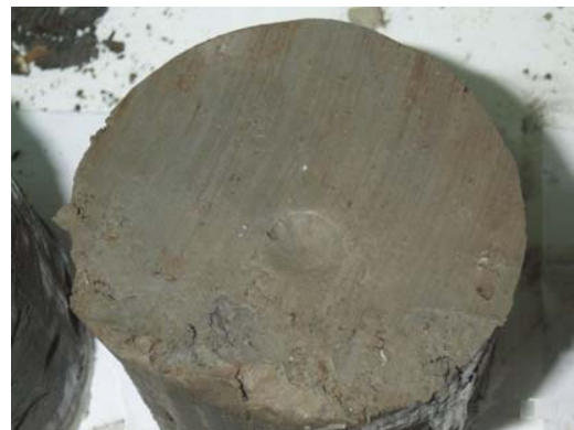
Figure 5. The fabric of a shear zone in highly fissured sheared tectonized clay shales: a) schematic representation; b) a specimen taken from the shear zone found at the base of the Masseria Marino mudslide
