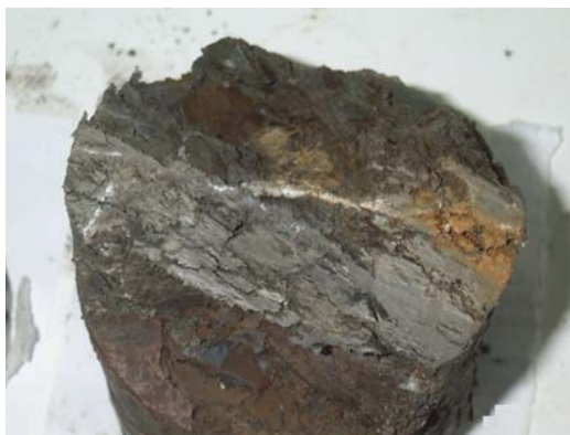
Figure 2. The fabric of highly fissured sheared tectonized clay shales: a) schematic representation; b) a specimen taken from the Masseria Marino clay shale
