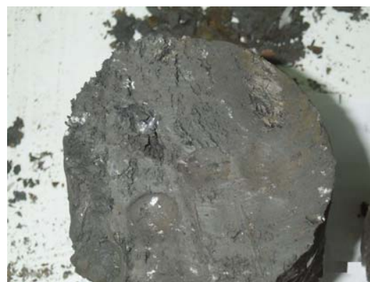
Figure 3. The fabric of a mudslide body in highly fissured sheared tectonized clay shales: a) schematic representation; b) a specimen taken from the Masseria Marino mudslide
