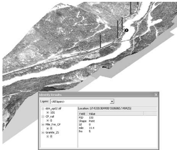
Figure 5: Spatial representation of rock fall frequency and orthorectified airphotos “draped” on a TIN surface.
