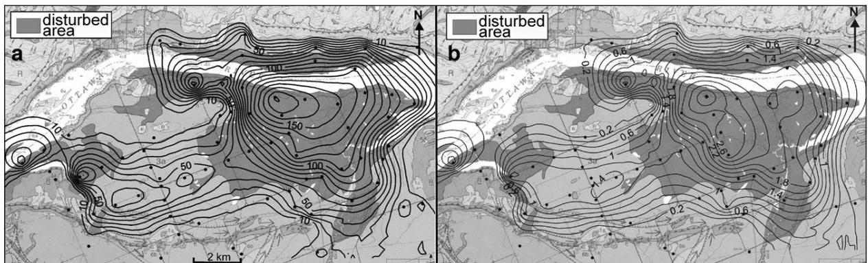
Figure 7 a) Overburden thickness map of the Lefaivre area from combined water-well and seismic reflection soundings. Contours in metres. Note correlation between "disturbed" ground and thick overburden. b) Fundamental resonance period variations derived from 2-way shear wave reflection travel times to bedrock. Contours in seconds. (after Benjumea et al. 2003)
