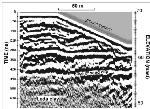
Figure 5. GPR profile across stable edge of the Bourget paleochannel showing sand cap over Leda clay. Although electrical methods indicated that the clay has been leached, the base of the sand cap is below the channel floor, so no landslide hazard exists at this site.
