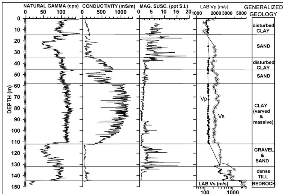
Figure 11. Example of geophysical logs for GSC borehole JA4. Holocene sediments have very low shear wave velocities in contrast to the higher Vs of the basal Pleistocene materials.
