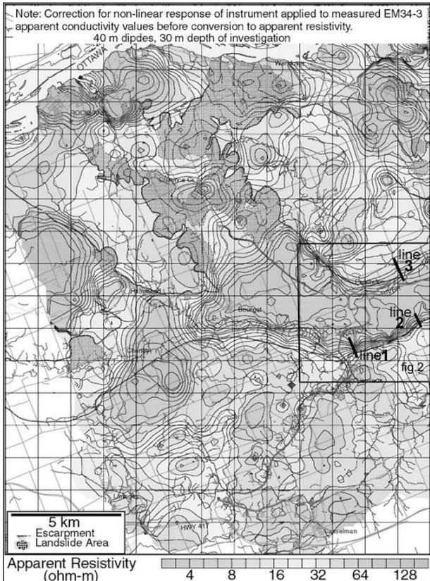
Figure 2. Average soil resistivity (from ground surface to a depth of 30 m) in the Bourget area. Constructed from EM-34 conductivity soundings at 800 m intervals along roads. Courtesy of T. Calvert. Location of figure 3 and lines of figure 4 are indicated.
