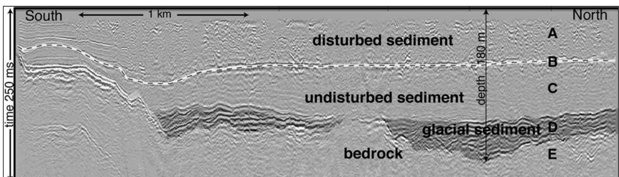
Figure 8. P wave seismic section across the Lefaivre basin. Unit A is disturbed sediment with poor record. Line B is a strong reflector that is interpreted to be the base of disturbance over most of the section. (after Benjumea et al. 2003.)
