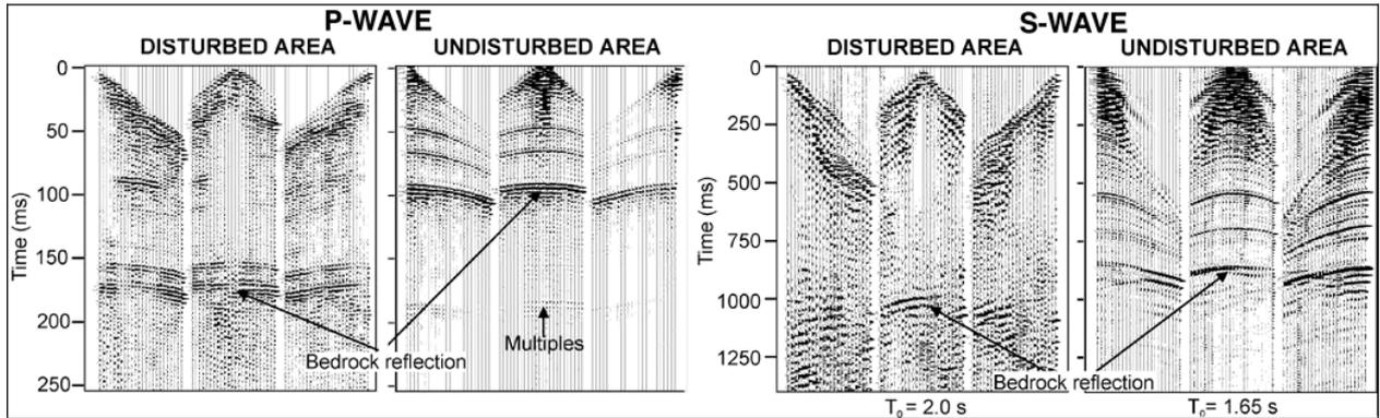
Figure 6. Example P and S wave reflection field recordings for a 24 channel seismic array for two sites in the Lefaivre area showing reflections from stratigraphy within the overburden as well as from the bedrock surface (after Benjumea et al. 2003). The fundamental resonance periods for the sites are computed as  $T_0 = 2 \times$  the two-way S-wave travel time to the bedrock surface. S wave reflection quality is adversely affected by ground surface disturbance.
