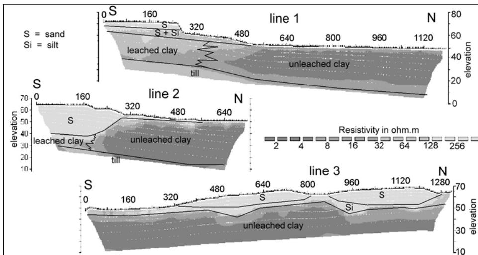
Fig. 4. ERI modeled with topography. Geological interpretation shown. Courtesy of T. Calvert.
