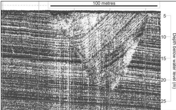
Figure 9. Single channel, high-resolution seismic profile of a rotated block of marine sediments. Detailed profiles across the feature show that the glide plain is spoon shaped and overall plane view is elliptical and measures about 100 x 200 m. VE: 4x.
