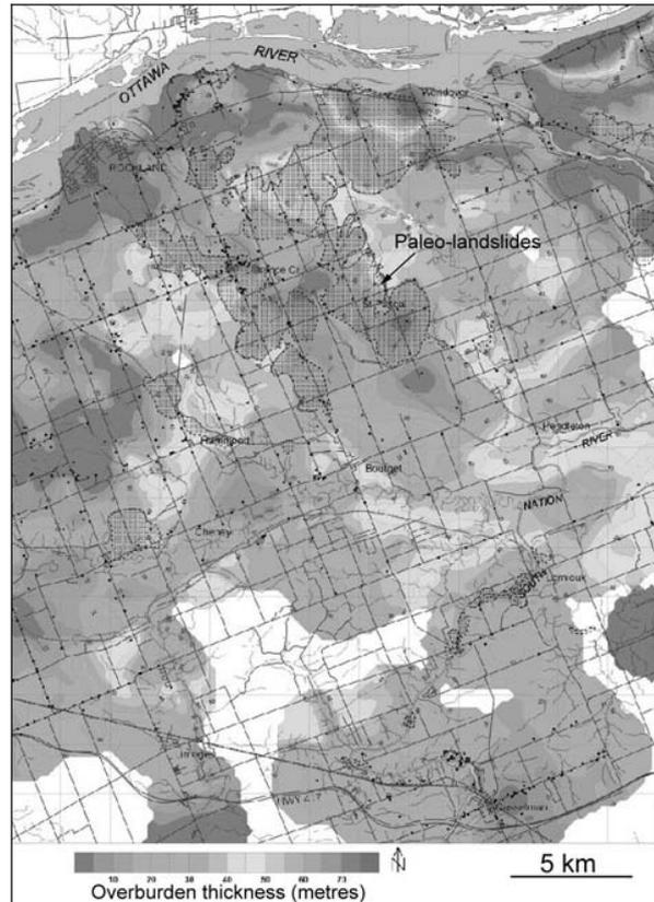
Figure 10. Map of overburden thickness for the Bourget area developed from a combination of water-well records and P wave refraction and reflection data.
