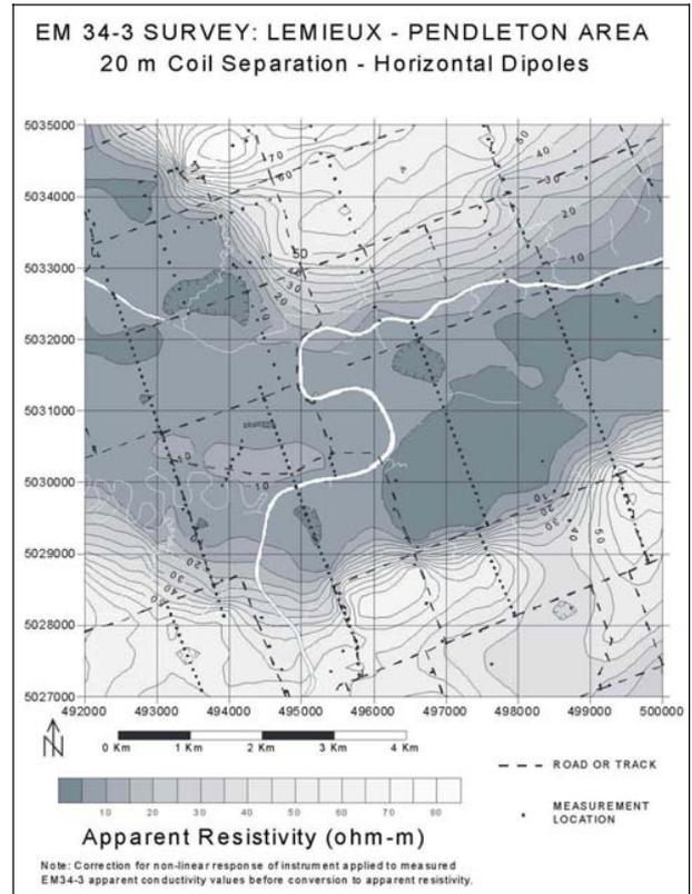
Figure 3. Average soil resistivity to a depth of 15 m. Low values are associated with stable Leda Clay. Higher values correlate with the presence of a sand cap and low saline (leached) clay conditions.
