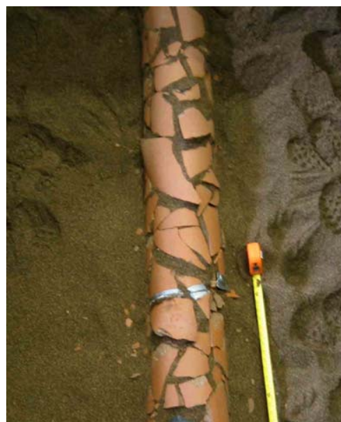
Figure 6. Photograph showing broken clay fragments from Test 3.
