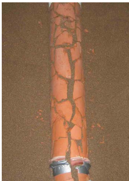
Figure 5. Photograph showing broken clay fragments from Test 2.
