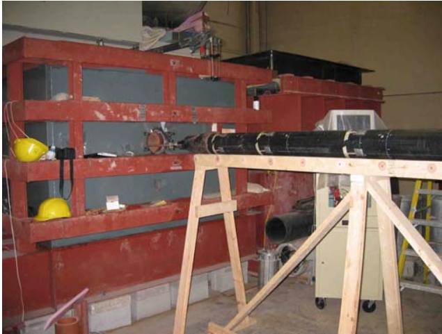
Figure 3: Steel tank, burst head and HDPE pipe prior to the experiment (from Lapos et al. 2004)
