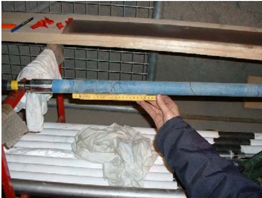
Figure 7. Original fracture traces on impression packer
