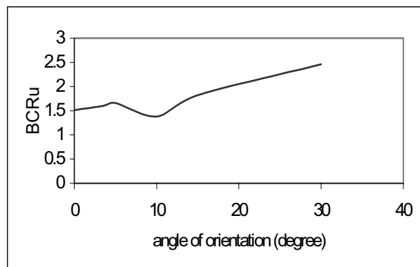
Figure 7. Variation of ultimate BCR_u for strip footing against reinforcement orientation
