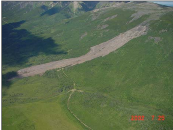
Figure 4. The Pink mountain landslide – a 2 km long rock slide – debris avalanche that achieved remarkable spreading and thinning through the undrained loading of entrained rock slide debris.
