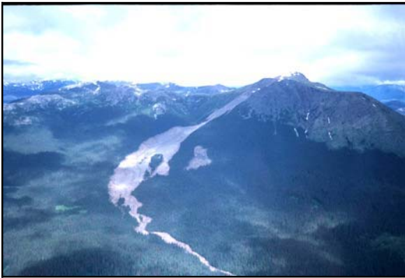
Figure 6. The Harold Price rock slide - debris flow (June 28, 2002) involved permafrost at its head. The smaller landslide to the right is a catastrophic earth spread that occurred in 1999.
