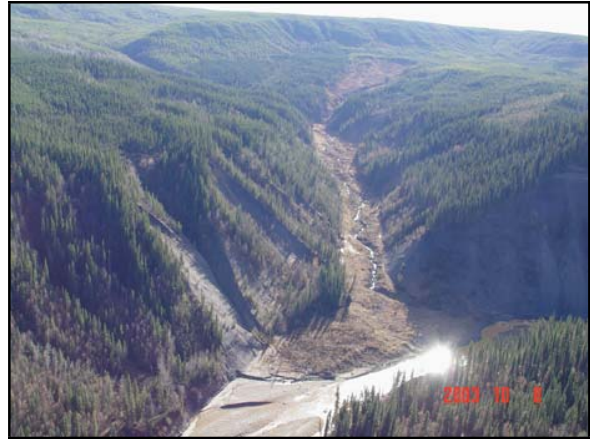
Figure 7. The Buckinghorse area of northeastern BC has reported sporadic permafrost and large rapid earth flows, such as this one which is 1.75 km long on a gradient as low as 3^\circ .
