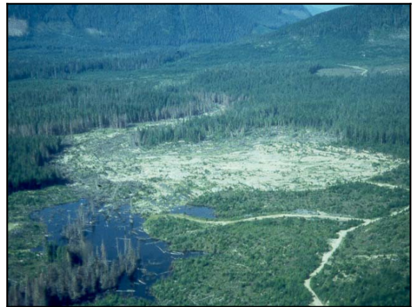
Figure 5. The Mink Creek earth flow-spread involved quick clays and occurred in glaciomarine sediments near Terrace, BC.
