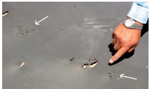
Figure-3: Photograph of a chemically attacked geomembrane
