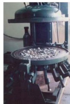
Aggregate puncture testing (CEMAGREF, FR)
