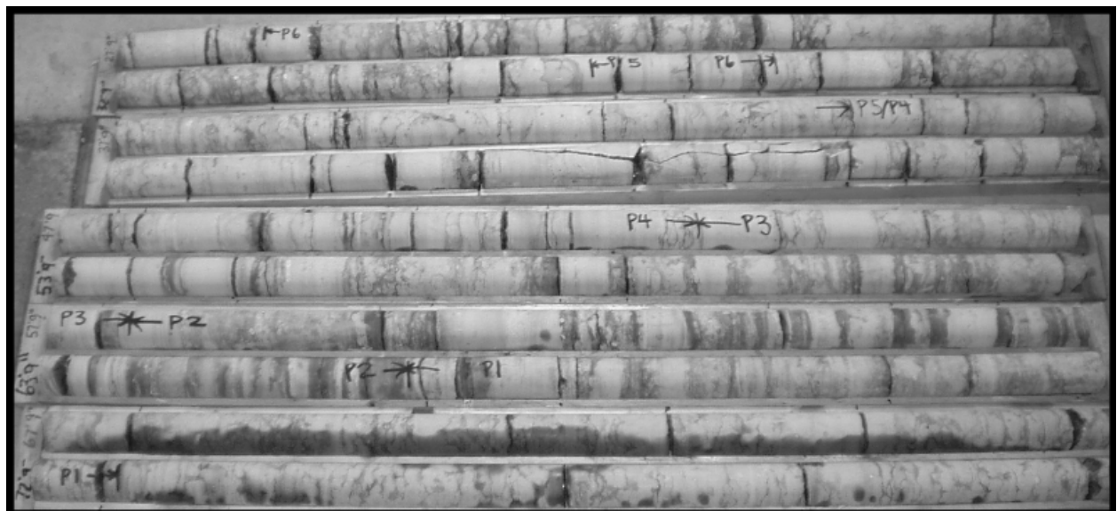
Figure 4. Photograph showing recovered core. Top of bedrock corresponds to the upper left, while the borehole bottom is at the bottom right. Hydraulic testing intervals (each 2.3 m in length) are identified directly on the core using the designation P1 (deepest) to P6 (shallowest).
