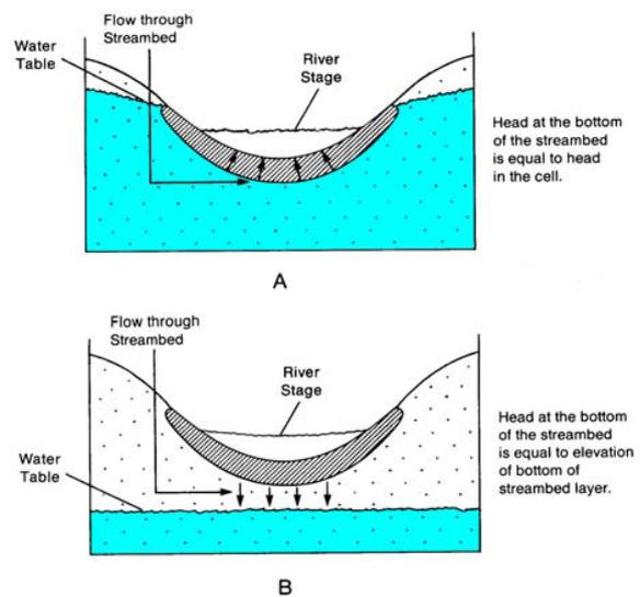
Figure 5: Stream-aquifer interaction processes. A = Discharge from ground to river. B = Recharge from river to ground
