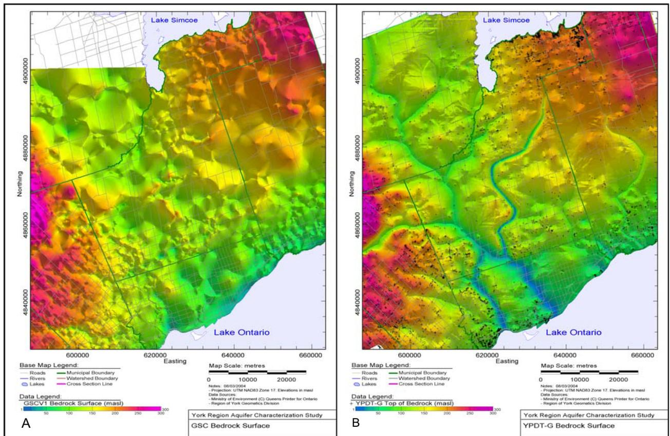
Figure 3: Comparison of unconstrained (left) and constrained (right) bedrock surface.
