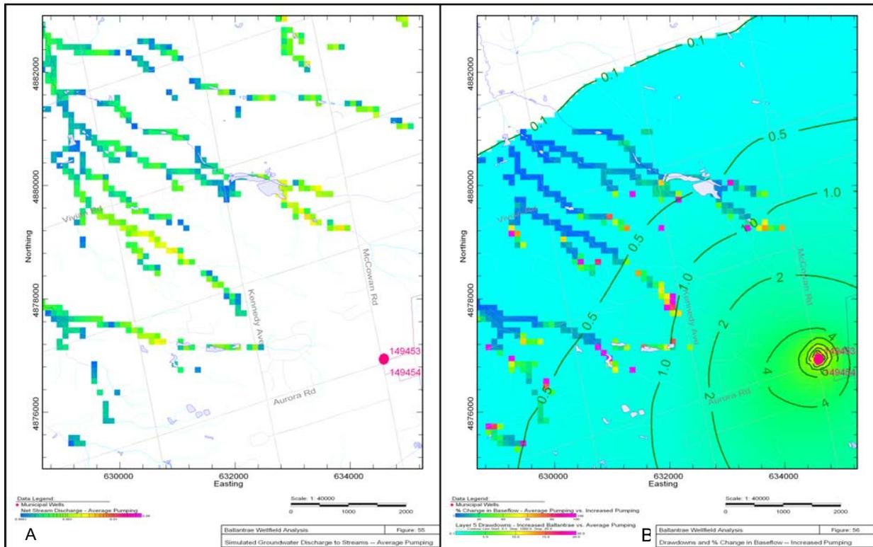
Figure 7: (A) Stream baseflow, (B) Percent change in baseflow due to pumping.
