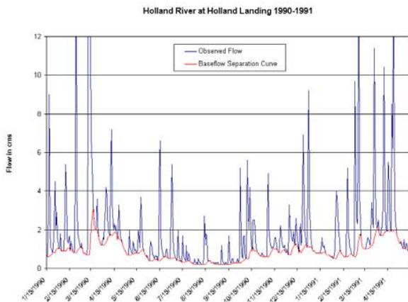
Figure 6: Baseflow separation estimates (red line) from total observer flow (blue line).
