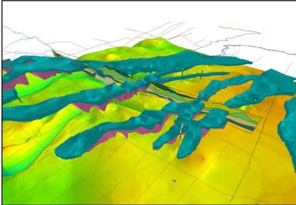
Figure 4: 3D view of tunnel channel deposits overlying bedrock surface (3D window size approximately 20 km).
