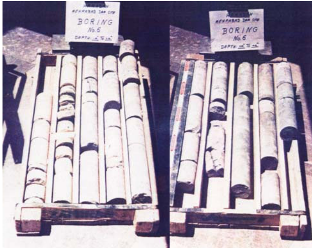
Figure 4. The cores of the borehole which are bored at the dam axis, from left to right (Mahab Ghodss, 1996)
