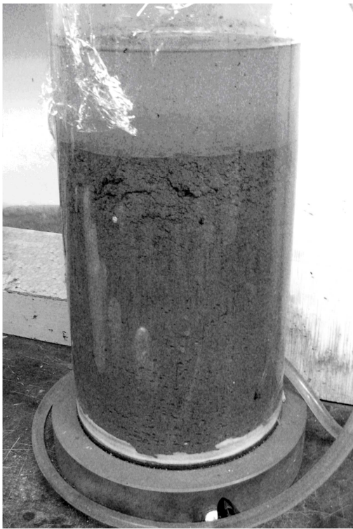
Figure 7. Flocculated tailings in the compressibility standpipe test
