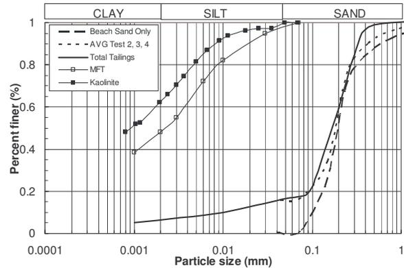
Figure 1. Typical grain size distributions for various oil sands tailings streams.
