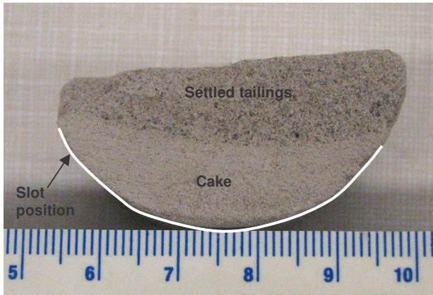
Figure 10. Cross section photo of the filter cake formed during Test 2.
