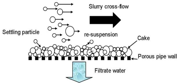
Figure 2. Schematic of cross flow filtration (modified from Ripperger and Altmann, 2002).
