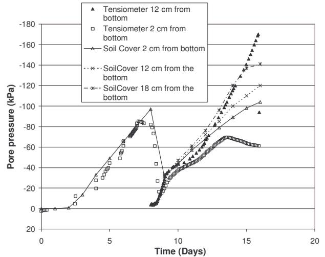
Figure 8 Matric suctions (negative pore pressure) measured and modelled during sequential deposition in the small-scale test on the Toromocho tailings
