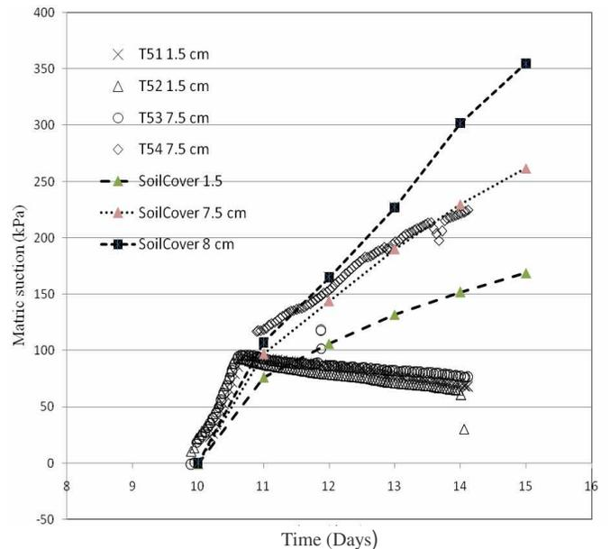
Figure 9 Matric suctions measured and modelled in second layer after deposition in large scale test.
