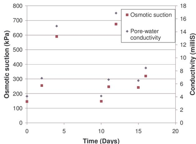
Figure 10 Evolution of pore-water conductivity and osmotic suction in the top 1 cm of the tailings in large scale test
