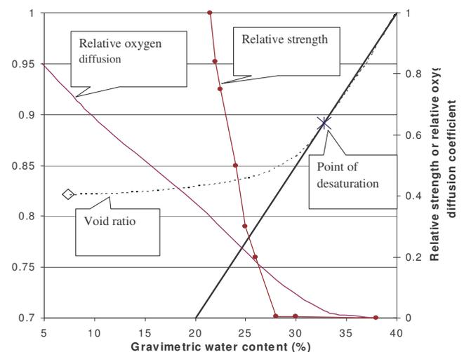
Figure 1. Shrinkage curve of paste tailings and associated geotechnical and geoenvironmental parameters (modified from Simms *et al.* 2007)
