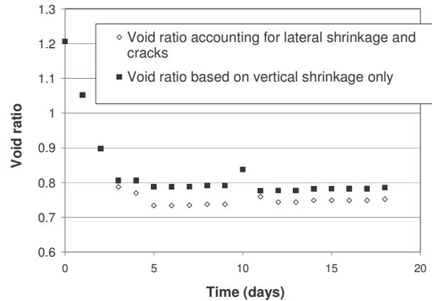
Figure 5 Volume change in large scale test
