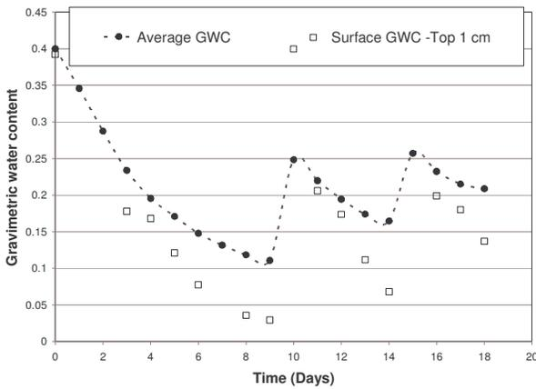
Figure 6 Average and surface gravimetric water contents in large scale test
