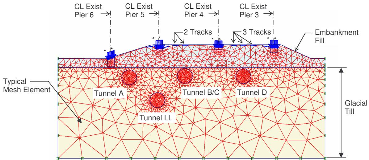
Figure 2. Typical Cross Section of Finite Element Model at Honeywell Street Bridge
