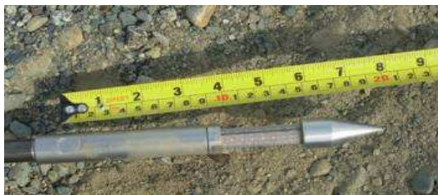
Figure 3. Extension pulled back to open the sampling section which is covered with fine screen mesh.
