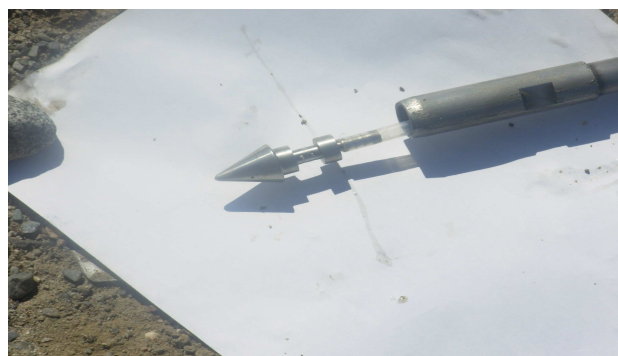
Figure 4. Tip (with gas inlet holes) linked to a fluoropolymer tube that runs through the driving extension
