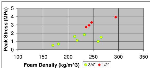
Figure 3: Foam Density vs. Peak Stress for cylinders tested at and installed into gravel at -15°C
