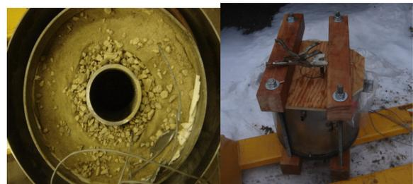
Figure 5: A pile ready for foam injection
