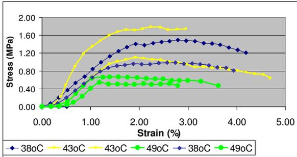
Figure 2: -15°C 3/4" aggregate prepared at different chemical preheat temperatures
