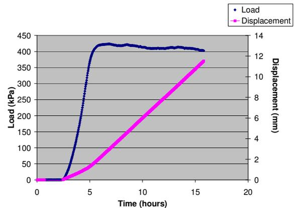
Figure 9: Pile Load 7 (mobilized stress only)
