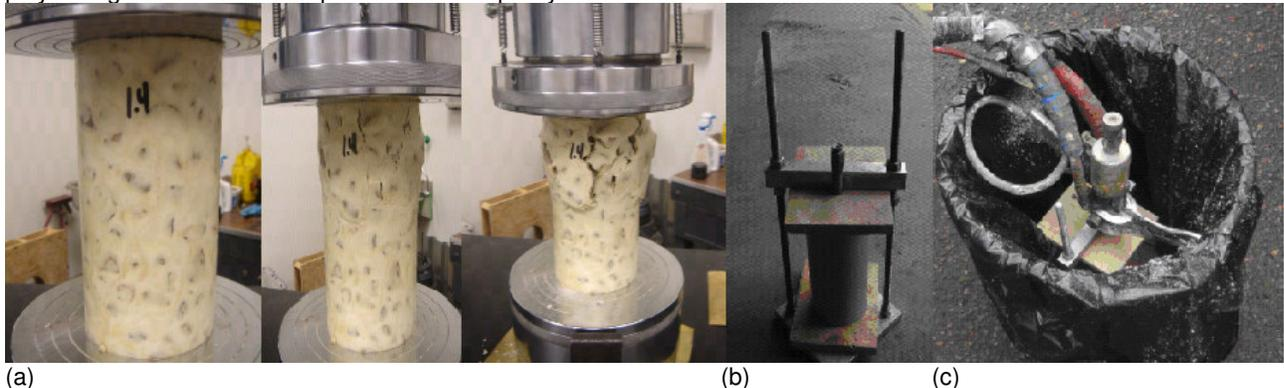
Figure 1: Polyurethane Concrete Cylinders: a) Unconfined Compressive Strength testing of sample 1.4. Frozen cylinder testing not shown. b) Injection frame clamping plastic cylinder filled with coarse aggregate. c) Injection gun clamped to cylinder. Red and Blue hoses contain chemical components with a third air line.
