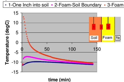
Figure 7: Thermal Effects of Pile Installation
