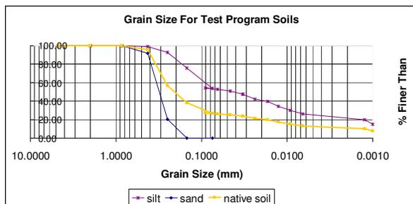
Figure 4: Test soil grain size distribution
