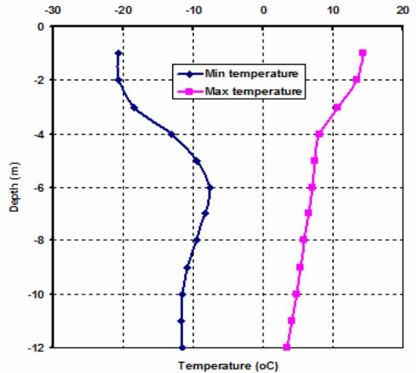
Figure 12. Trumpet of temperature of 5m-10m (3)) string at Face 1 of test pile 2 from the surface of test pile
