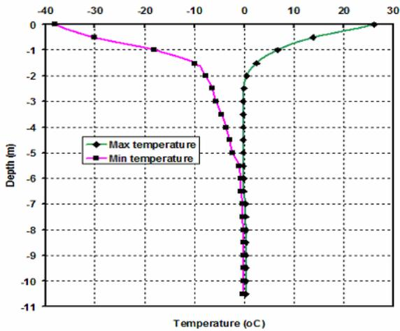
Figure 15. Trumpet of test pile 3 (covered pile) at center cross section
