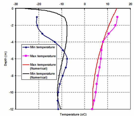
Figure 20. Comparison between field data (5m-10m(3)) with numerical modeling with air permeability K = 1.10<sup>-7</sup> m<sup>2</sup>
