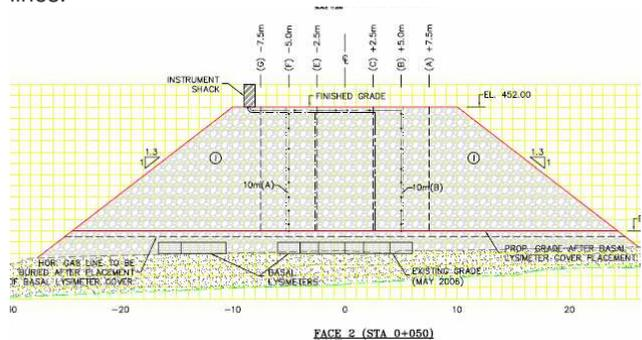
Figure 4. Typical cross section (Face 2) of Type 1 and Type 2 piles
