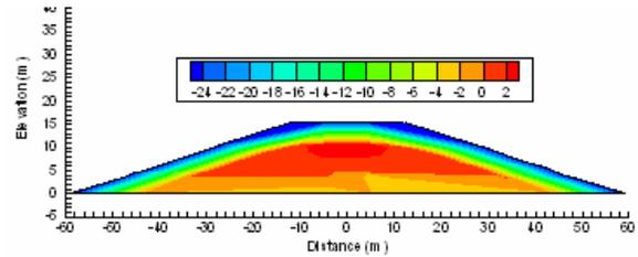
Figure 16. Contour temperature of test pile 3 (covered pile) at face 2 March 18, 2008
