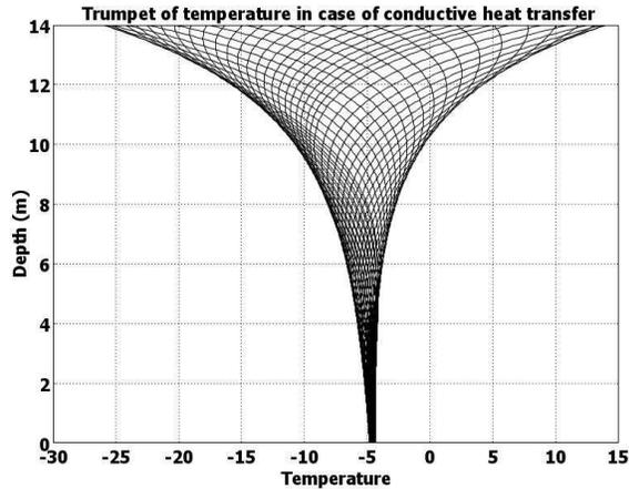
Figure 25. Trumpet of temperature in case of conduction or low values of air permeability ( $K < 3.10^{-9} \text{ m}^2$ )
