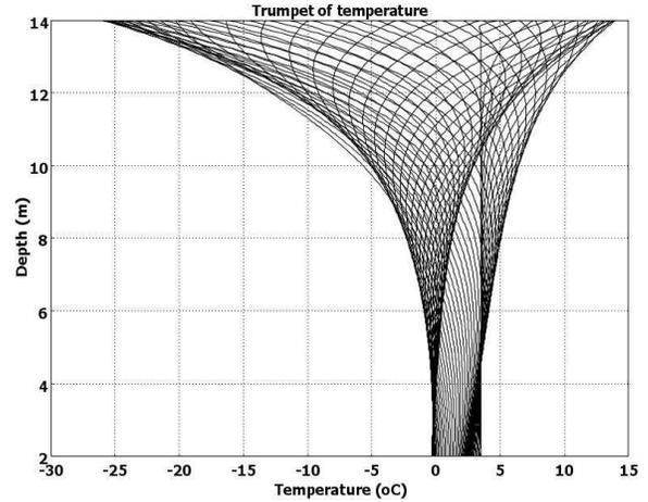
Figure 19. Trumpet of temperature at line shifted 5m from center line 650days after construction with K = 3.10<sup>-9</sup> m<sup>2</sup>
