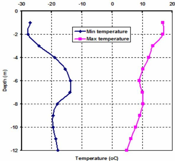
Figure 10. Trumpet curve of temperature of one vertical (2m-5m (3)) string at Face 1 of test pile 1 from the surface of test pile and shifted 5m to the right from centre line.
