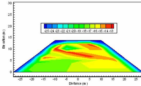
Figure 14. Temperature contour of test pile 2 at face 4 on March 18<sup>th</sup> 2008.
