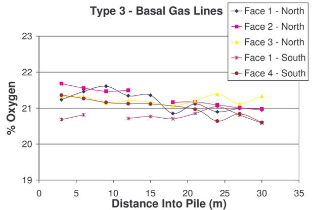
Figure 18. Concentration of O<sub>2</sub> and of test pile 2 (Rich Amos, 2007)
