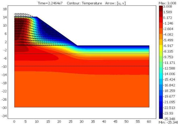
Figure 21. Temperature profile at the first winter with  $K = 1.10^{-7} m^2$
