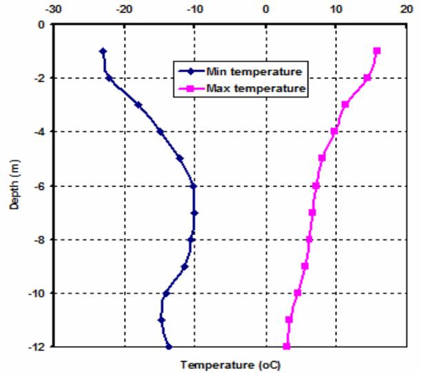
Figure 11. Trumpet of temperature of 5m-10m (6)) string at Face 1 of test pile 2 from the surface of test pile
