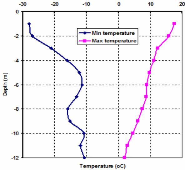
Figure 9. Trumpet curve of temperature of one vertical (2m-5m (2)) string at Face 1 of test pile 1 from the surface of test pile and shifted 5m to the left from centre line.
