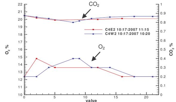
Figure 17. Concentration of O<sub>2</sub> and CO<sub>2</sub> at Face 4 of test pile 3 (Rich Amos, 2008)
