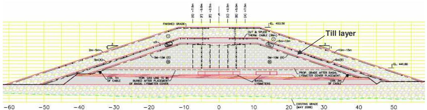
Figure 6. Typical cross section (Face 3) of Type 3 (covered pile) with locations of thermistors and other instruments
