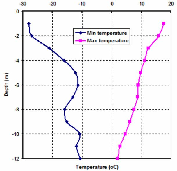
Figure 8. Trumpet curve of temperature of one vertical (2m-5m (2)) string at Face 1 of test pile 1 from the surface of test pile and shifted 5m to the left from centre line.
