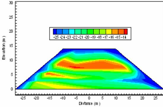
Figure 13. Temperature contour of test pile 1 at face 4 on March 18<sup>th</sup> 2008.
