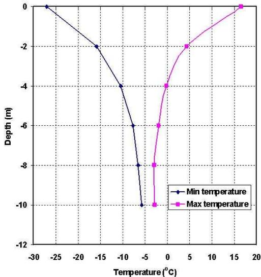
Figure 7. Trumpet curve of ground temperature at Diavik mine site.
