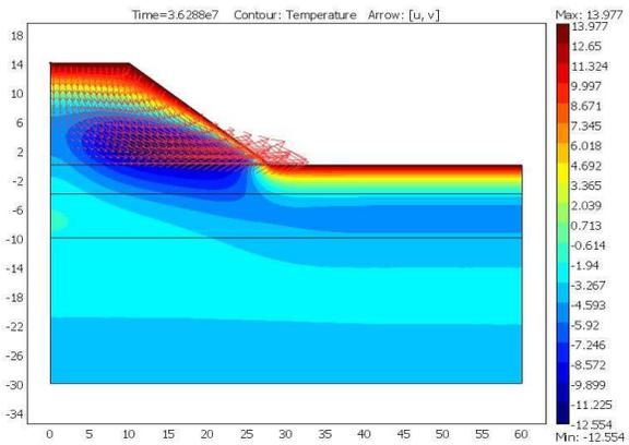
Figure 22. Temperature profile at the first summer with  $K = 1.10^{-7} m^2$
