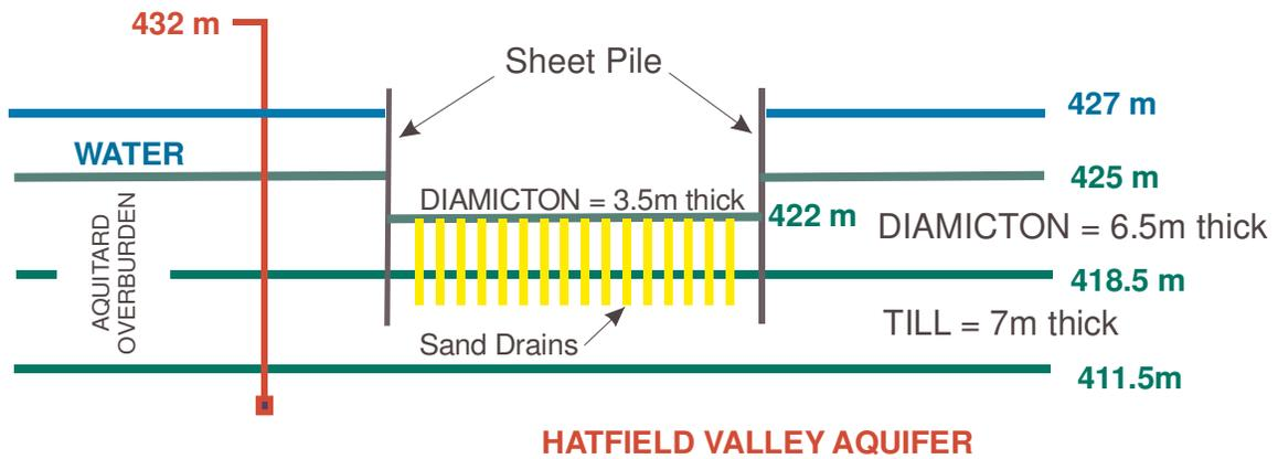
Figure 4: Schematic representation of cofferdam and sand drain configuration.
