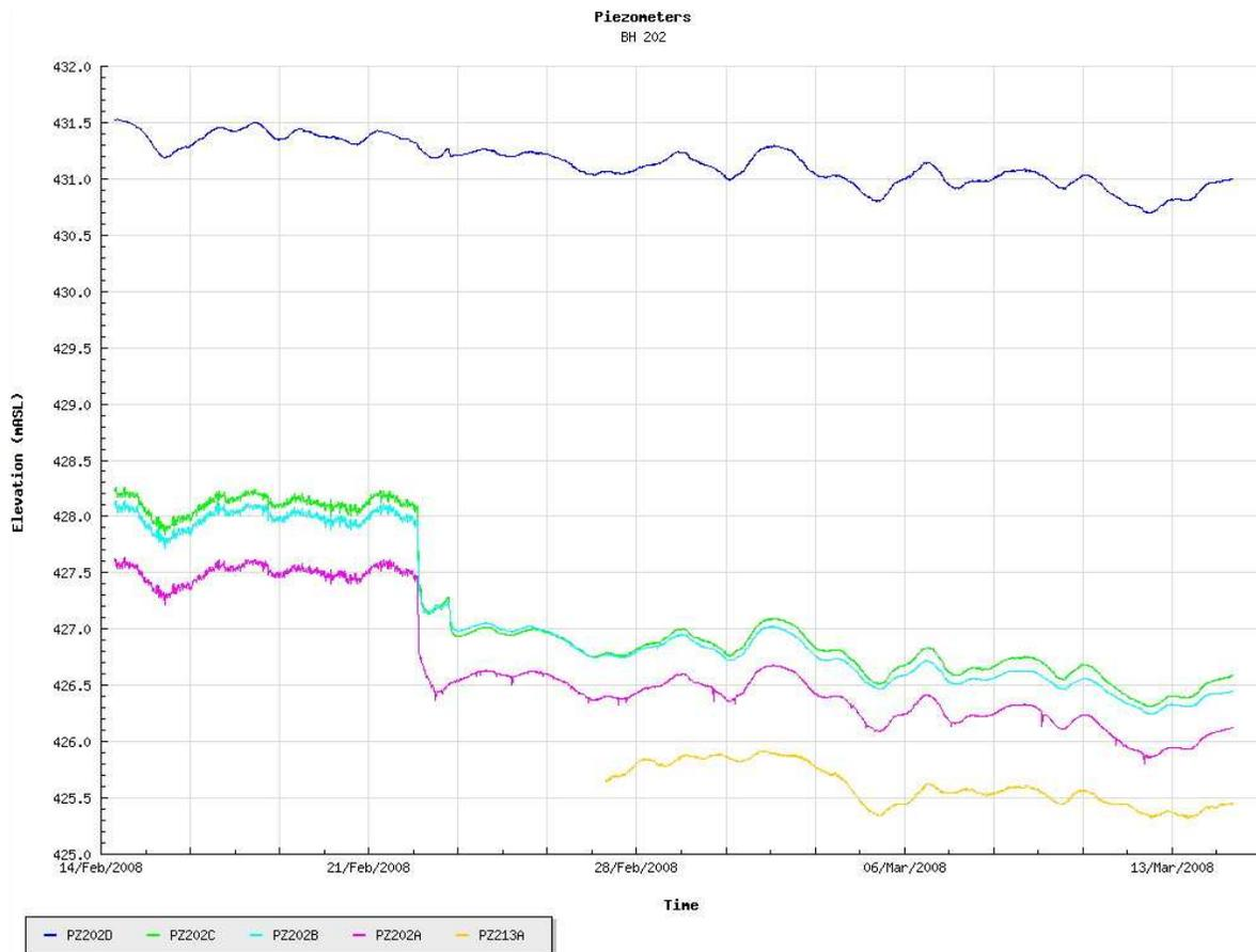
Figure 11: Results of sand drain response
