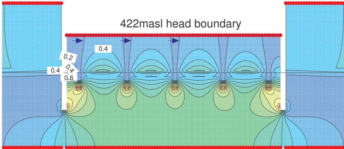
Figure 5: Gradient contours for 4.5 m spacing of sand drains within the cofferdam, following excavation of 3 m into the Diamicton.
