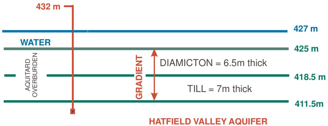
Figure 3: Schematic representation of the geological input parameters for the analysis.
