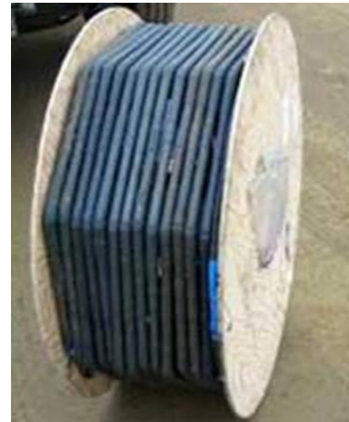
Figure 5. SAA on spool (104 m array shown) (Abdoun and Bennett 2008).
