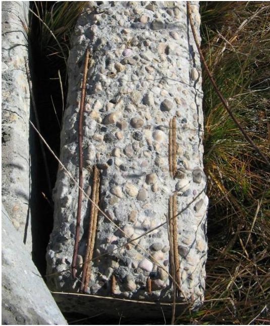
Figure 3. Picture of the worn underside of concrete-tie. This tie is a typical example of the ties removed from between mile 101.4 and 102.1 in October 2007.
