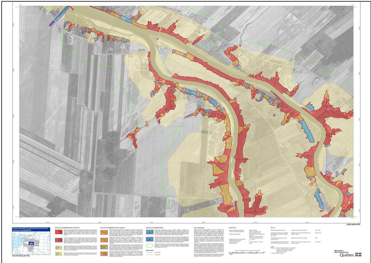
Figure 3: Example of a landslide susceptibility map
