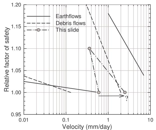
Figure 7. Relation between relative factor of safety for earthflows and debris slides taken from Bonnard and Glastonbury 2005, shown with estimates for the landslide in this study.
