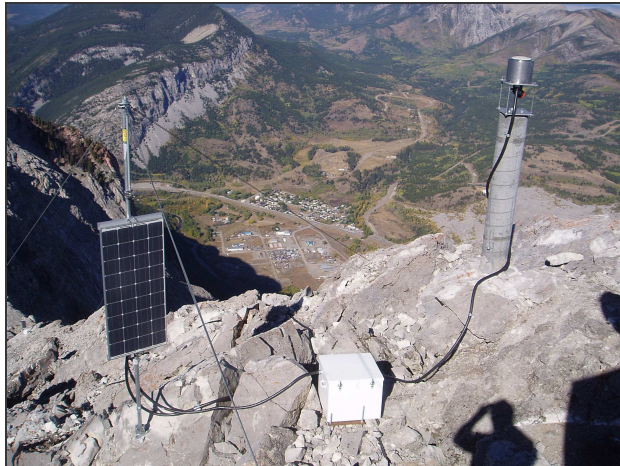
Figure 2. Typical Turtle Mountain GPS Station showing the antenna (right), battery (centre) and solar panel (left)
