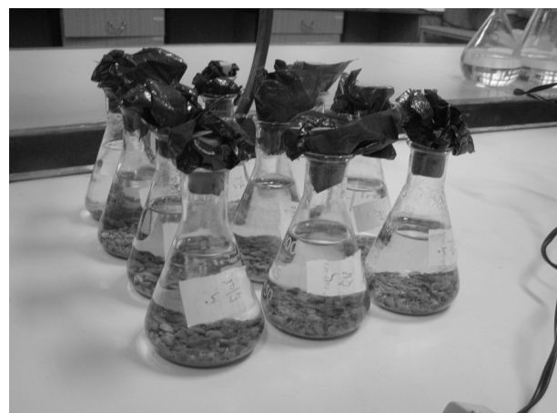
Figure 4. Batch Adsorption tests setup
