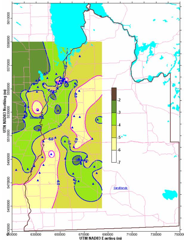
Figure 9 Log-K (m/s) Distribution in Carbonate Aquifer
