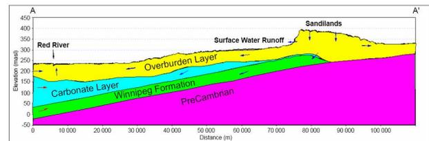
Figure 3 A – A' Geological Cross-Section (The location is shown on Fig.1)
