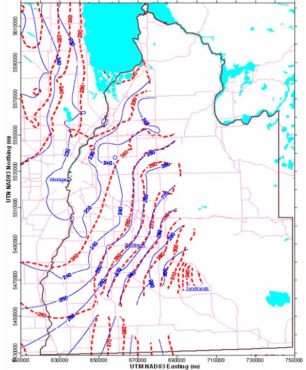
Figure 13 Groundwater Level in Carbonate Aquifer (Notes: blue contours – observed groundwater level in 2005, dashed red lines – simulated steady state groundwater level)
