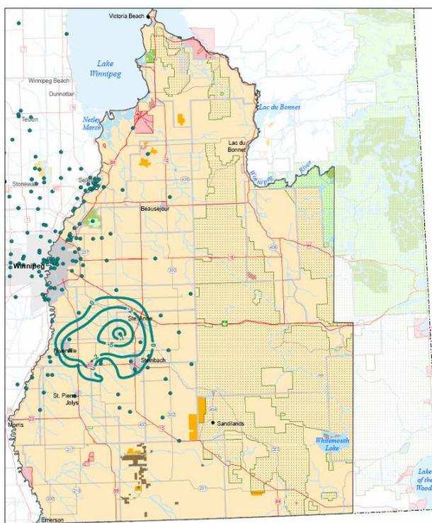
Figure 15 Negative Drawdown in Carbonate Aquifer between 2005 and 1991
