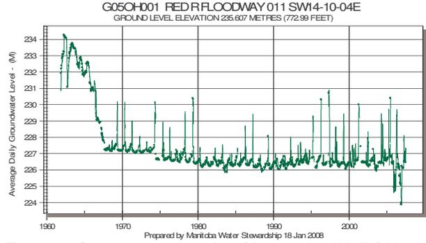
Figure 6 Groundwater Level in Observation Well OH001
