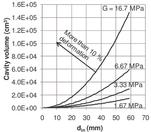
Figure 8 : Filter zone volumes and riser pipe diameters resulting in  $dV_{cavity}/dV_{pipe} = 10\%$  for different undrained shear modulus.
