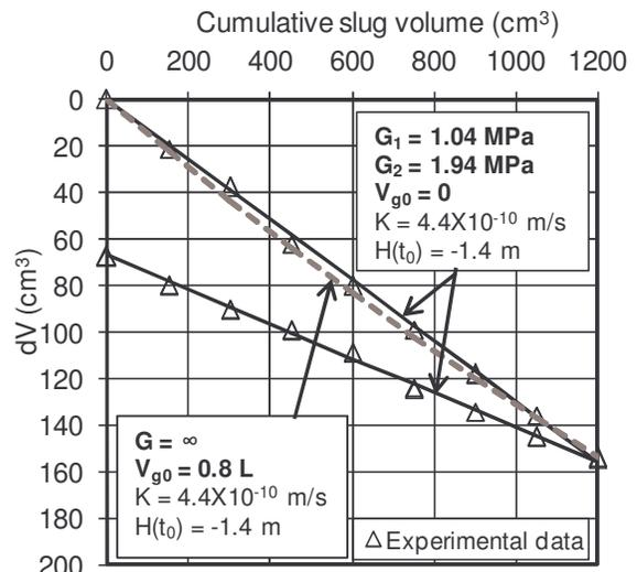
Figure 4. Comparison between test results for the second observation well and numerical simulations with cavity deformation or air storage effect scenarios
