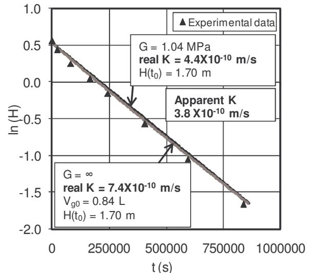
Figure 5: Plot of  $\ln(H)$  vs.  $t$  for numerical simulations and experimental data resulting in an apparent  $K$  value of  $3.8 \times 10^{-8}$  m/s.
