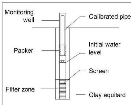
Figure 2. Using a calibrated pipe to evaluate cavity and gas volume change
