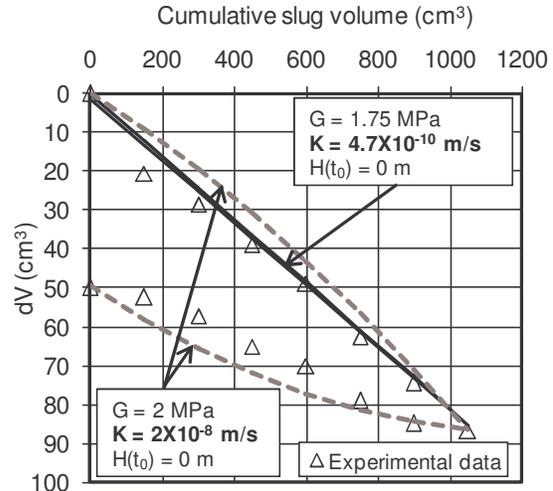
Figure 3. Comparison between test results for the first observation well and two curves obtained numerically for two K values.
