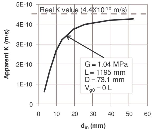
Figure 7: Apparent hydraulic conductivity as a function of riser pipe diameter.
