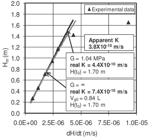
Figure 6: Velocity graph for numerical simulations and experimental data resulting in an apparent K value of  $3.8 \times 10^{-8}$  m/s.
