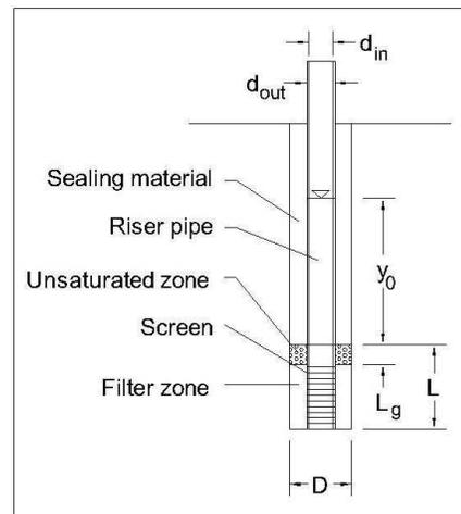
Figure 1. Symbols used in the demonstration
