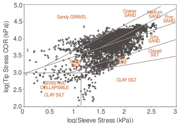
Figure 1 - Fellenius and Eslami (2000) CPT profiling chart showing the log of the tip stress (kPa) versus the log of the sleeve stress (kPa).
