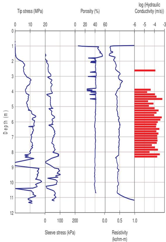
Figure 3 - Typical profiles of CPTu/SMR soundings and hydraulic conductivity measurements.
