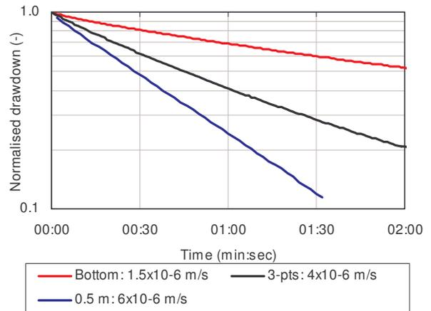
Figure 2 - Observed normalised drawdown as a function of time at observation well P6-362P for different pumping-surgings well development configurations. Hydraulic conductivity is proportional to the slope of the time-drawdown curve. Note that for the 0.5-m configuration over-pumping did not change the slope of the time-drawdown curve (not shown).
