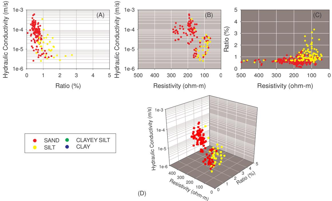
Figure 5 - (a), (b) and (c) Scatter-plots of hydraulic conductivity versus CPTu/SMR parameters. (d) 3D graph of hydraulic conductivity versus *ratio* (tip/sleeve) and resistivity. The vertical resolution is 15 cm and the measurement scale is 15 cm. Sediment textures are based on the Fellenius and Eslami (2000) profiling chart (see Figure 1).
