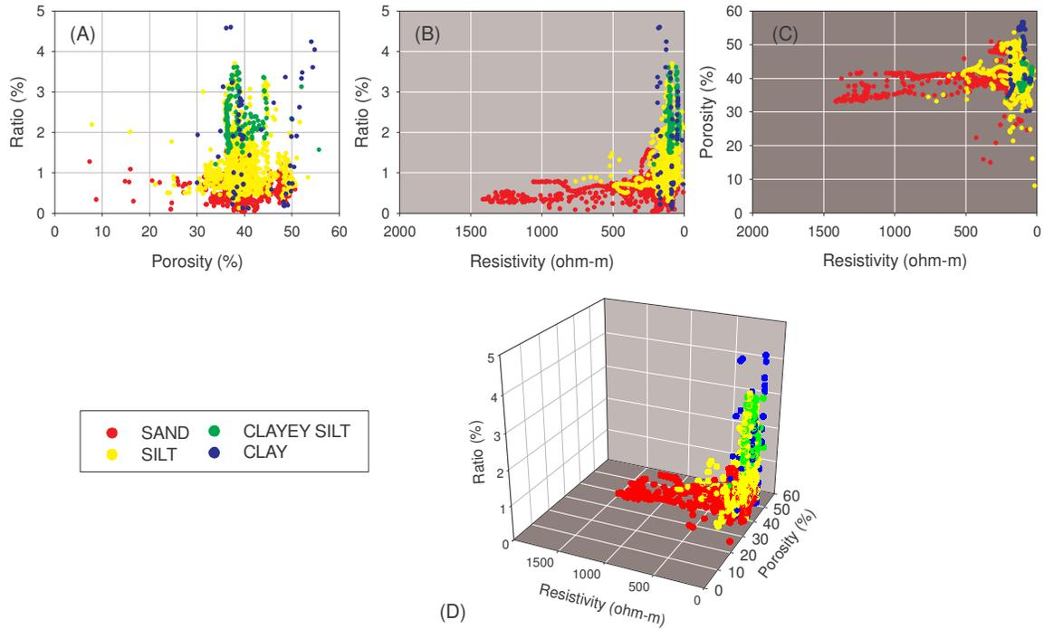
Figure 4 - (a), (b) and (c) Scatter-plots of CPTu/SMR measurements. (d) 3D graph of *ratio* (tip/sleeve) versus resistivity and porosity. The vertical resolution is 3 cm and the measurement scale is 9 cm. Sediment textures are based on the Fellenius and Eslami (2000) profiling chart (see Figure 1).
