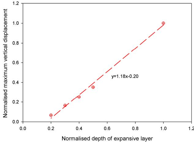
Figure 7. Normalised depth of expansive layer versus normalised maximum vertical displacement at the basement foundation.
