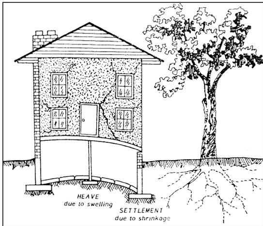
Figure 1. Damage to houses caused by ground movements of swelling soils (Domaschuk, 1986).
