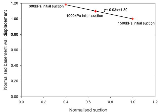
Figure 5. Normalised suction versus normalised wall displacement.
