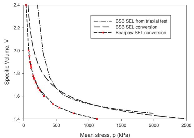
Figure 2. The Swell Equilibrium Limit (SEL) plotted in specific volume versus mean stress space.
