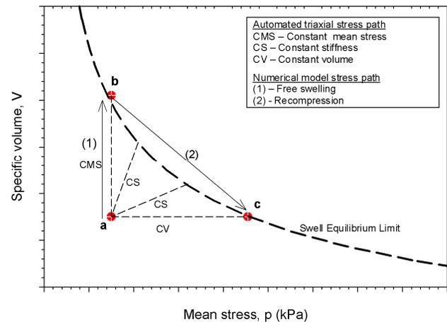
Figure 3. Boundary conditions applied in automated triaxial infiltration test and numerical model in specific volume versus mean stress space.
