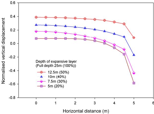
Figure 6. Normalised vertical displacement at basement foundation with respect to the vertical heave that occurs at 25m depth of expansive soil.
