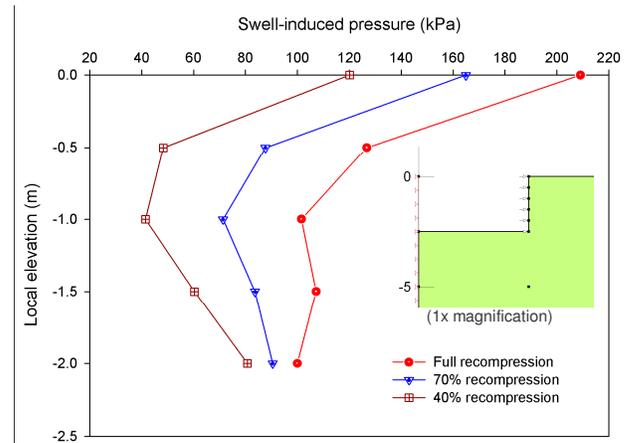
Figure 8. Swell-induced pressure on the basement wall with varying degree of recompression.
