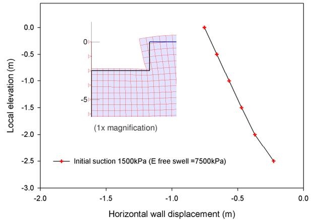
Figure 4. Horizontal wall displacement due to ponding at basement foundation.
