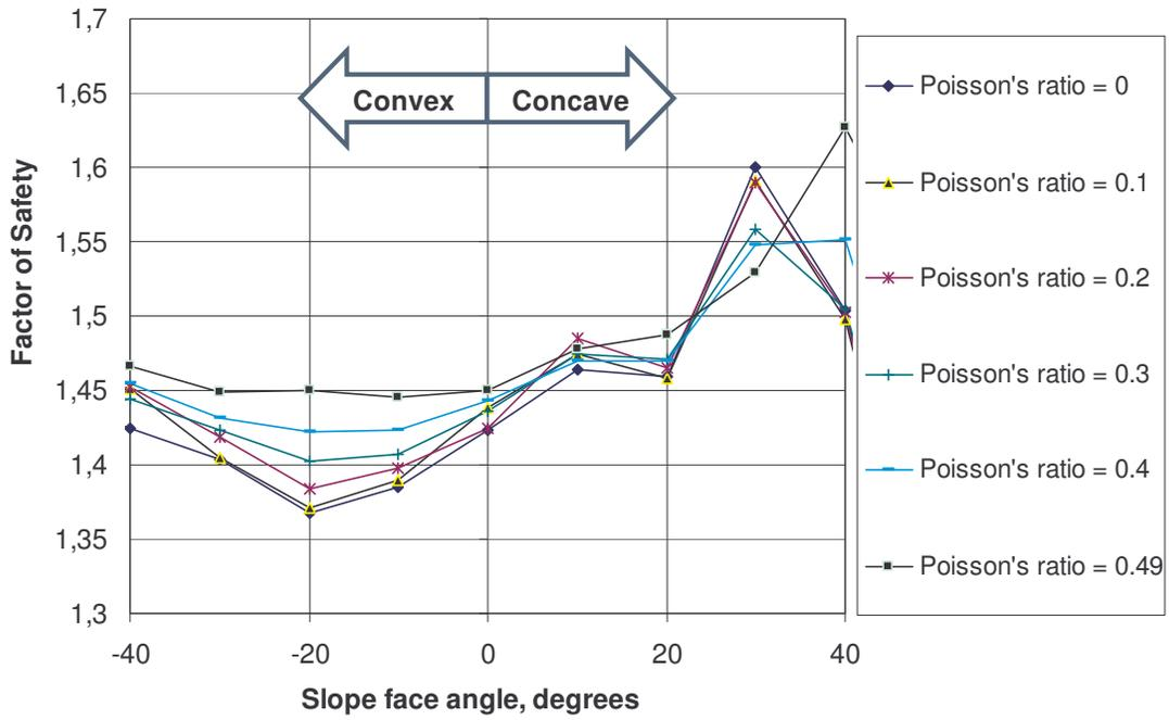
Figure 5. Three-dimensional factor of safety for various scenarios.
