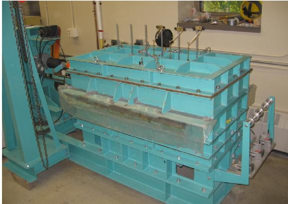
Figure 1: Large Scale Direct Shear Apparatus
