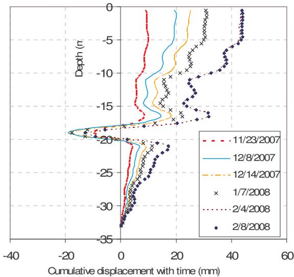
Figure 3. Lateral displacements measured at BH-1
