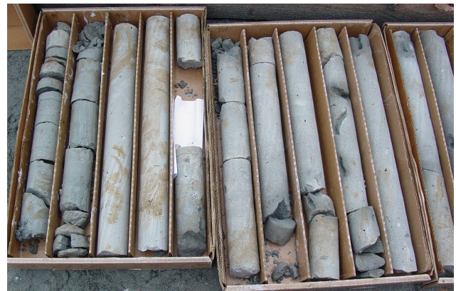
Figure 2. Soilcrete cores extracted from Brightwater East test section at three column interstice
