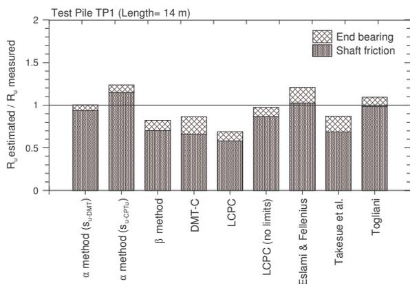
Figure 5. Estimated/Measured ultimate load capacity for the test pile TP1
