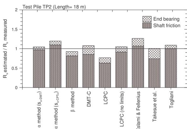
Figure 6. Estimated/Measured ultimate load capacity for the test pile TP2
