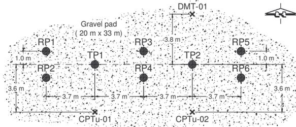
Figure 1. Test pile layout and location of CPTu and DMT soundings
