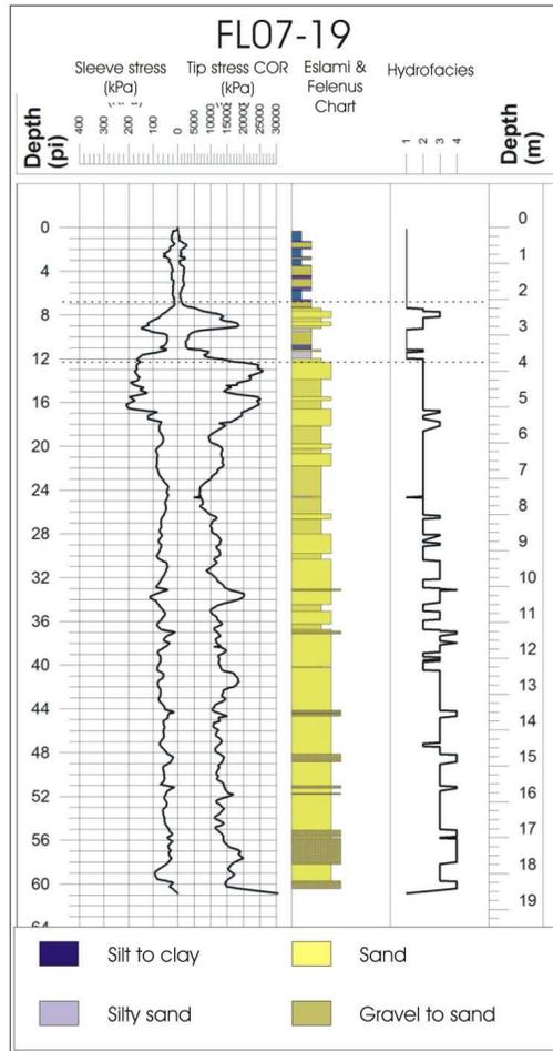
Figure 5. Stratigraphic and hydrofacies interpretation from the CPT borehole based on Eslami and Fellenius chart. (Width of Stratigraphic column is proportional to grain size)
