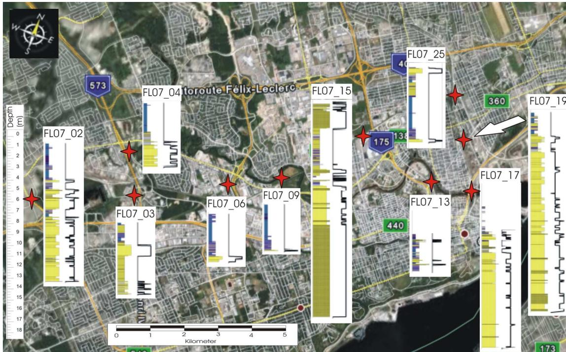
Figure 6. Stratigraphic and hydrofacies of the Quebec City delta based on CPT and borehole interpretation. (Stratigraphy column width is proportional to grain size, see Figure 4 legend)
