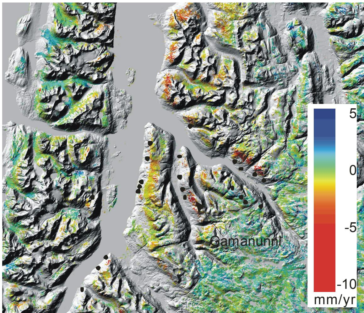
Figure 3. InSAR results from the Lyngen peninsula and Kåfjord. The area shown is 65 x 55 kilometres. Black dots represent areas visited in the field during 2007. The average velocity from 1992 to 2000 is shown in mm/yr. Details of the Gamanjunni rockslide are shown in Figure 4.
