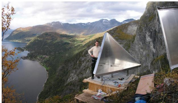
Figure 5. Artificial corner reflector installed on a moving block on the north side of Tafjord. After installation, the reflectors are covered to prevent snow accumulation.
