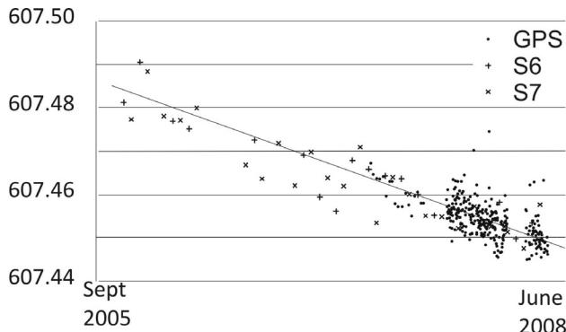
Figure 6. Elevation (metres) vs time as derived from permanent GPS and InSAR for the centre of the Åknes landslide. ENVISAT data from S7 and S6 image modes were processed independently. Both GPS and InSAR datasets are affected by changing atmospheric conditions, but show an average vertical displacement of 13 mm/yr.
