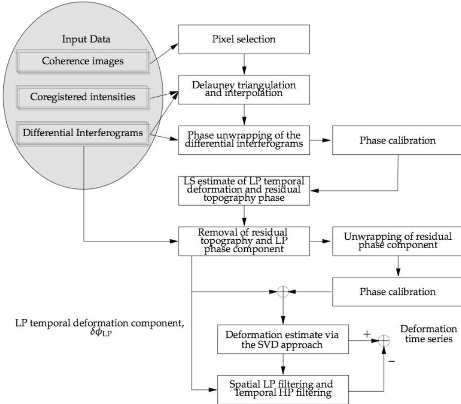
Figure 1. Flow chart showing the implementation of the small-baseline subset (SBAS) algorithm used in this study (Lauknes et al., 2005).
