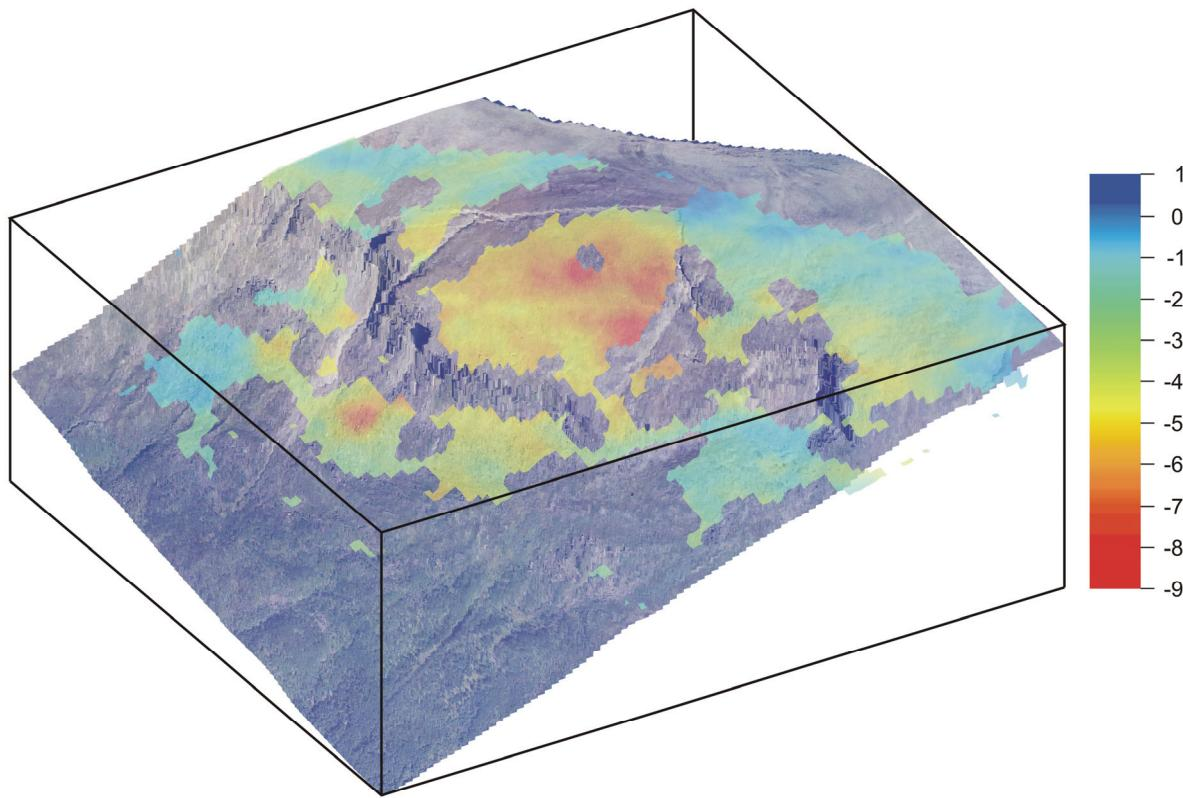
Figure 4. Gammanjunni rockslide is located in Troms County. The area shown in the figure is just over 2 kilometres on each side. The average velocity from 1992 to 2000 is shown in mm/yr.
