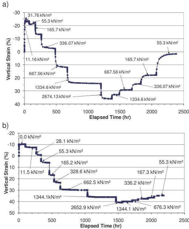
Figure 4. Vertical strain versus time graphs for a) representative test using distilled water (MN2) and b) representative test using 250 g/l CaCl<sub>2</sub> solution (JPM5).
