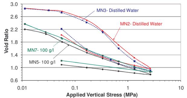
Figure 7. Void ratio versus log vertical stress plots for the distilled water tests (MN2 and MN3) and the 100 g/l CaCl<sub>2</sub> tests (MN5 and MN7).
