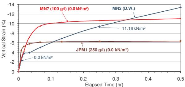
Figure 6. Vertical strain versus time graphs for test MN2 (distilled water), MN7 (100 g/l) and JPM1 (250 g/l) for the first 0.5 hours of initial swelling.
