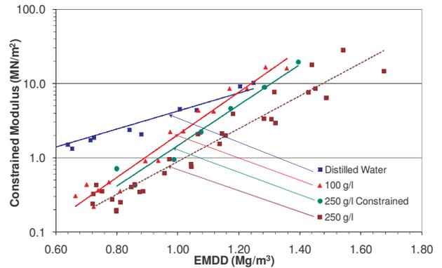
Figure 9. Constrained modulus versus EMDD for loading paths.
