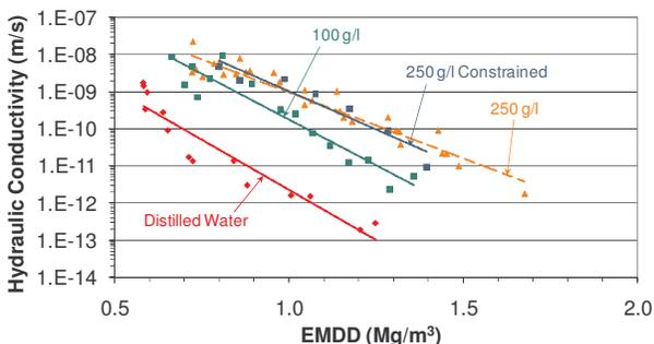
Figure 10. Hydraulic conductivity versus EMDD for loading paths.
