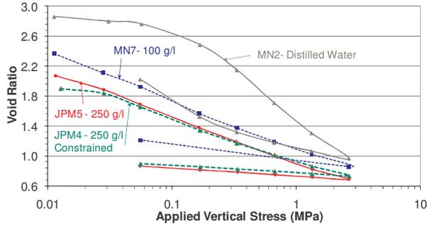
Figure 8. Void ratio versus log vertical stress plots for a distilled water test (MN2), a 100 g/l CaCl<sub>2</sub> test (MN7), a 250 g/l CaCl<sub>2</sub> test (JPM5) and the 250 g/l CaCl<sub>2</sub> constrained test (JPM4).
