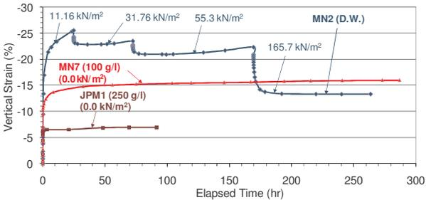
Figure 5. Vertical strain versus time graphs for tests HB6 and MN2 (distilled water), MN7 (100 g/l) and JPM1 (250 g/l) during initial swelling.
