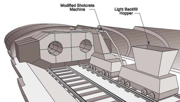
Figure 2. Remote Placement of Light Backfill Material.
