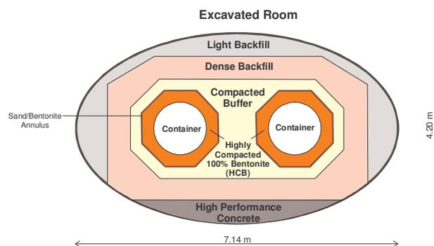
Figure 1. Third Case Study In-room Emplacement Geometry (after Gierszewski et al. 2004).
