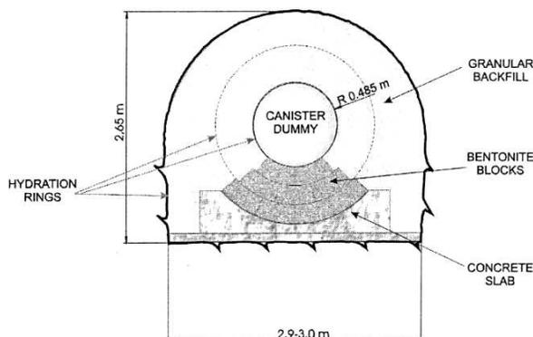
Figure 3. Configuration of the Mont Terri Engineered Barrier Experiment (Fuentes-Cantillana and Huertas 2002).
