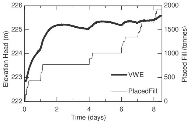
Figure 9. VW-E porewater pressure response and placed fill load vs. time
