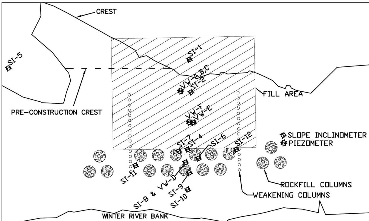
Figure 2. Layout of rockfill column test site
