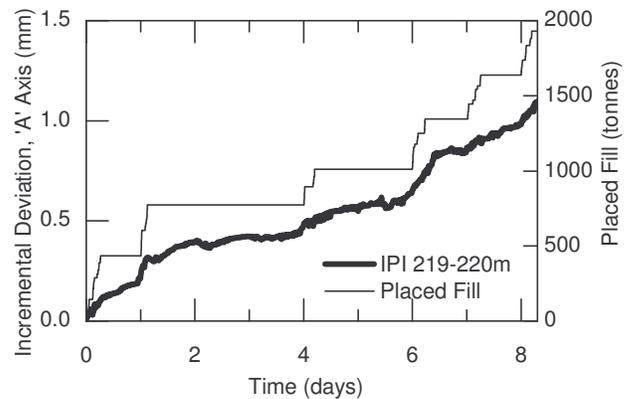
Figure 8. SI-8 IPI deviations and placed fill load vs. time
