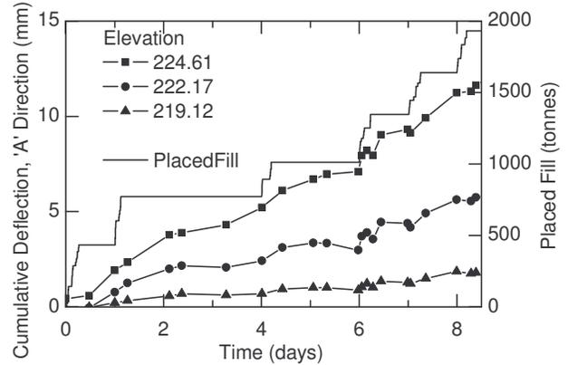
Figure 7. SI-7 displacements at three (3) depths and placed loading fill vs. time
