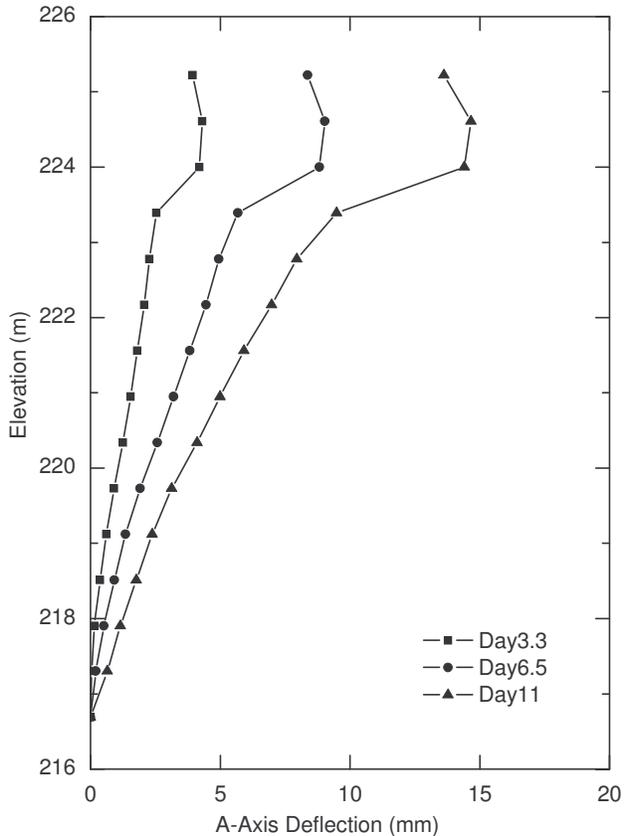
Figure 6. Deflections vs. depth as measured with a slope inclinometer. Baseline prior to test loading
