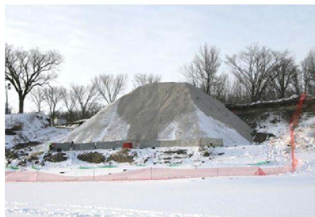
Figure 5. Rockfill Column research site during test loading
