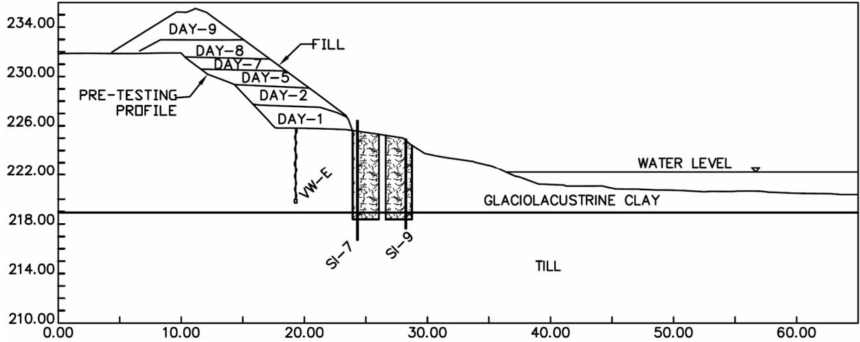
Figure 1. Cross section through centerline of rockfill column test site showing fill staging and select instrumentation
