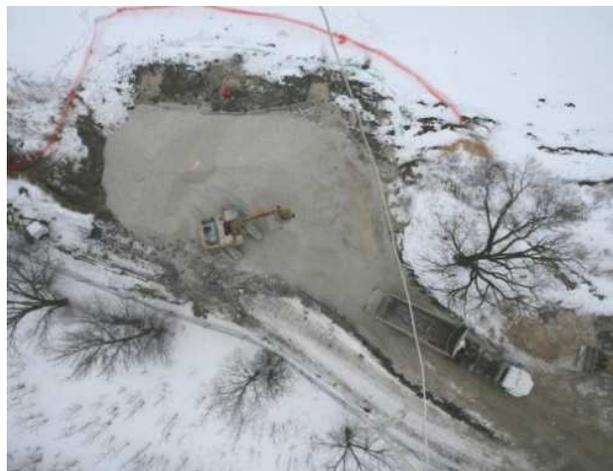
Figure 4. Aerial view of rockfill column research site during test loading with photo taken from tethered aerostat
