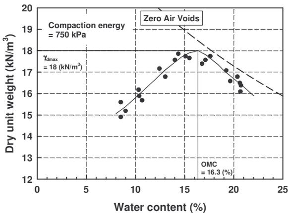
Figure 3. Compaction curve for Indian Head till
