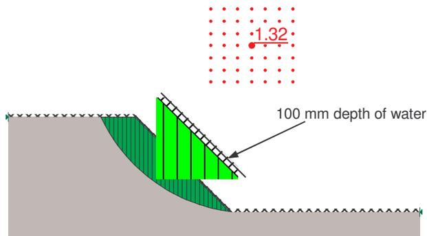
Figure 11. Stability analysis for ponding condition for saturated embankment
