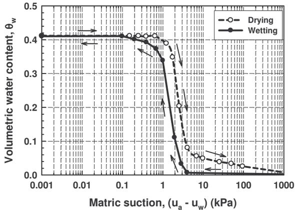
Figure 2. Hysteresis of soil-water characteristic curve (after Tami et al., 2004)
