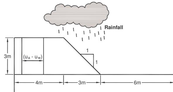
Figure 4. Cross-section of the embankment used in the present study
