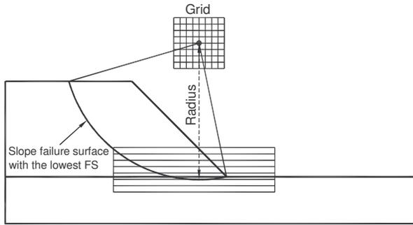
Figure 5. The grid and radius method of specifying trial slip surfaces
