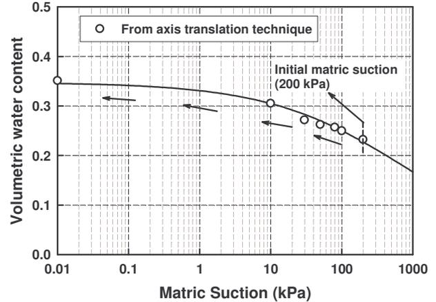
Figure 7. Wetting soil-water characteristic curve of the Indian Head till
