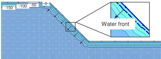
Figure 15. Pore-water pressure profile within embankment due to rainfall (40 mm/hour) at the moment of failure
