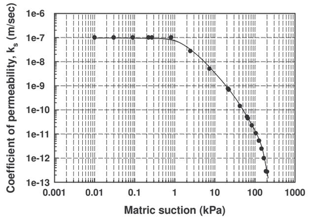
Figure 8. The variation of coefficient of permeability with respect to matric suction of glacial till
