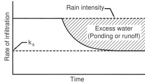
Figure 1. Variation of rate of infiltration with time (after Hillel, 1982)
