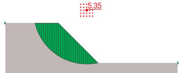
Figure 9. Stability analysis for saturated condition with  $\bar{C}U$  results ( $c' = 36.8$  kPa)
