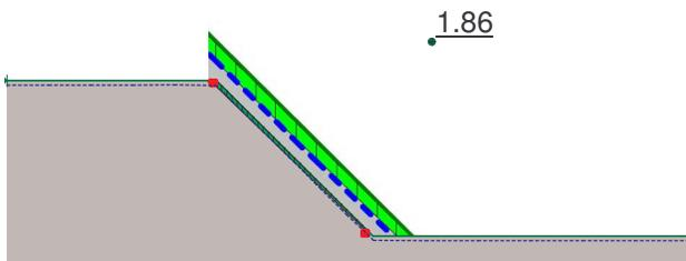
Figure 14. Long term stability analysis for unsaturated condition considering rainfall infiltration (Block method)
