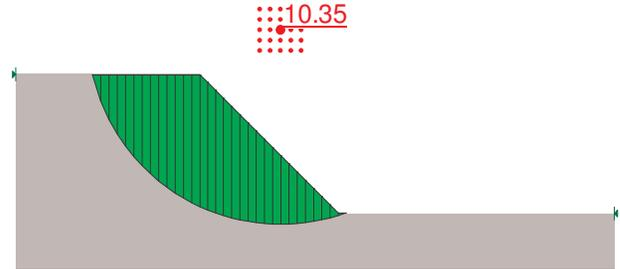
Figure 16. Short term stability analysis for unsaturated condition using IU results
