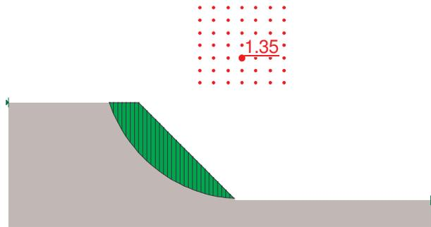
Figure 10. Stability analysis for saturated condition using CD results ( $c' = 5$  kPa)
