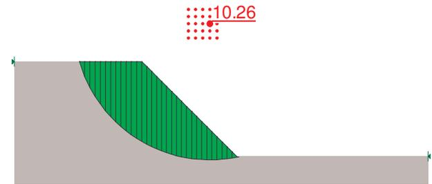
Figure 12. Long term stability analysis for unsaturated condition without rainfall infiltration
