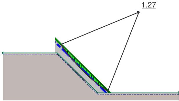
Figure 13. Long term stability analysis for unsaturated condition considering rainfall infiltration (Grid and radius method)
