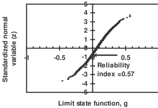
Figure 7. Reliability analysis results of non-liquefiable data using Youd et al. assessment method (CPT-liquefaction based data from Moss et al. 2006)
