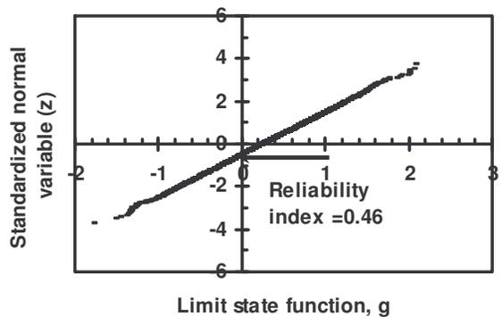
Figure 10. Reliability analysis results of non-liquefiable soils using data and assessment method from Moss et al. 2006
