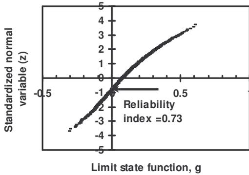
Figure 6. Reliability analysis results of liquefiable data using Youd et al. assessment method (CPT-liquefaction based data from Moss et al. 2006)
