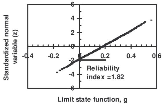
Figure 9. Reliability analysis results of liquefiable soils using data and assessment method from Moss et al. 2006
