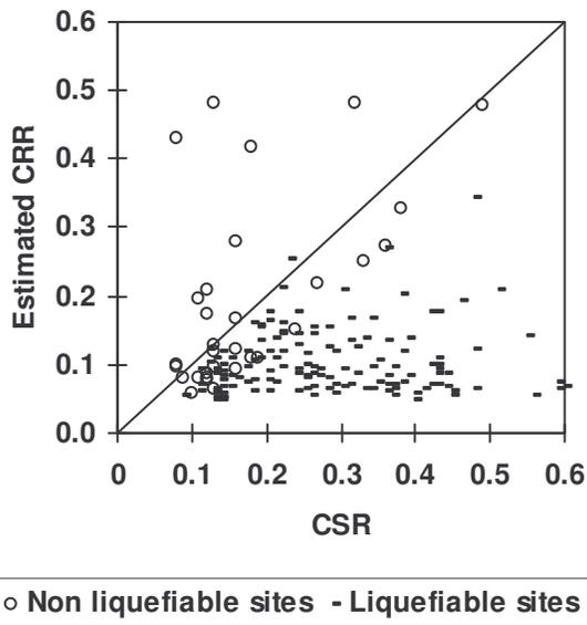
Figure 8. Comparison between CSR and estimated CRR using Moss et al. (2006) assessment method and database
