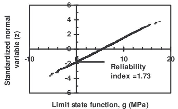
Figure 4. Reliability analysis results of non liquefiable data using Shibata and Teparaksa assessment method (CPT-liquefaction based data from Stark and Olson 2005)
