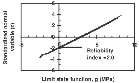
Figure 3. Reliability analysis results of liquefiable data using Shibata and Teparaksa assessment method (CPT-liquefaction based data from Stark and Olson 2005)
