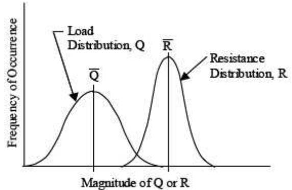
Figure 1a. Schematic of normally distributed load ( $Q$ ) and resistance ( $R$ )
