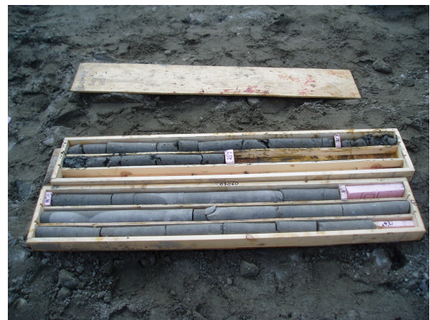
Photo 9- Coring of Jet-Grouted columns
