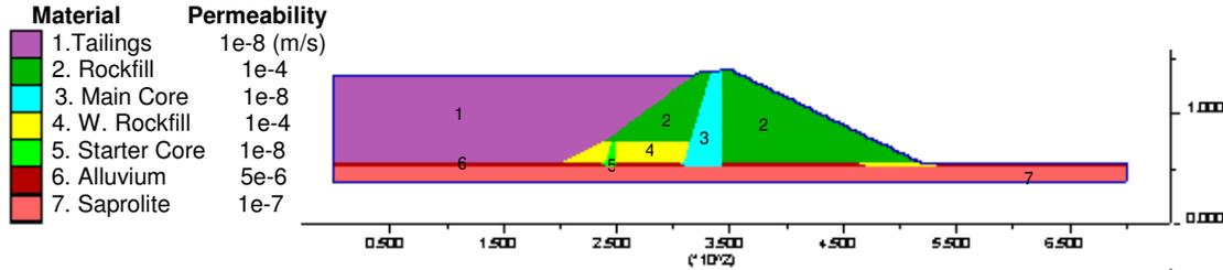
Figure 5. Various soil types and permeability values used in modeling.
