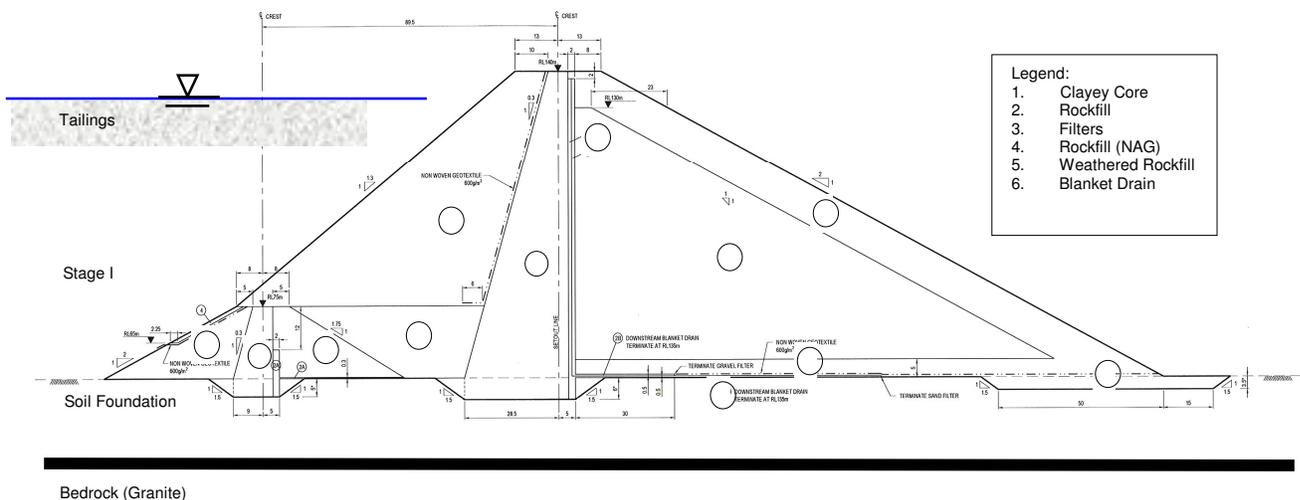
Figure 2. Typical maximum cross-section of Oxide tailings dam with different zones at closure stage.
