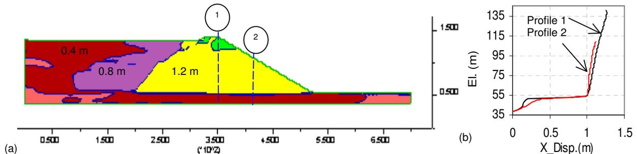
Figure 7. Dam-foundation deformation pattern, (a) x-disp. profile, (b) x-disp. profile at positions 1 and 2.
