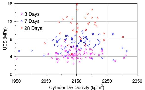
Figure 8. UCS versus dry density of cylinders
