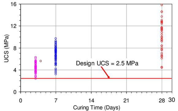
Figure 7. UCS versus curing time
