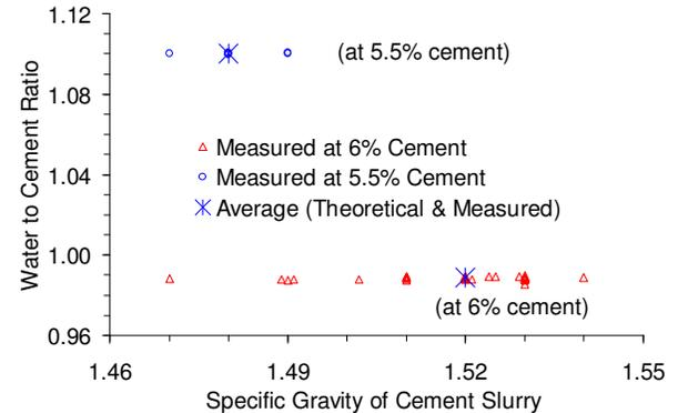
Figure 5. Water to cement ratio versus specific gravity of cement slurry
