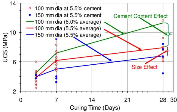
Figure 9. UCS of different CRF-cylinder sizes & cement content versus curing time
