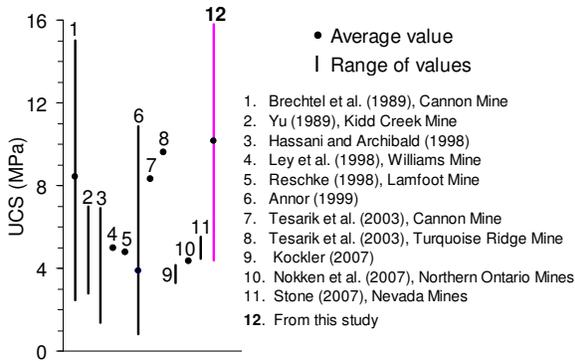
Figure 10. Laboratory UCS of (5.5 & 6% cement) CRF from this study compared with reported values
