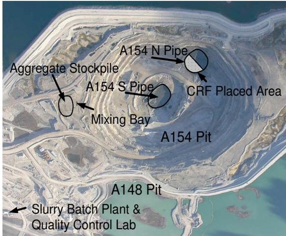
Figure 1. Location of CRF placement area at A154 pit (after DDMI, 2005)
