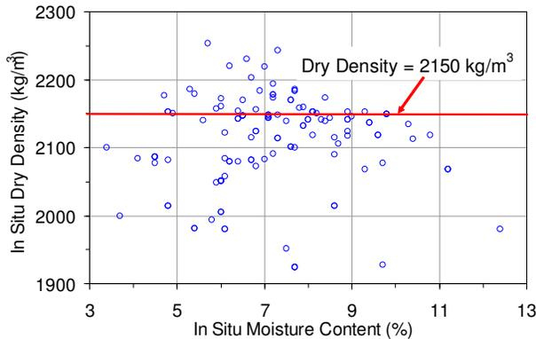
Figure 6. In situ dry density versus moisture content
