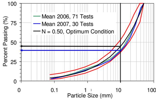
Figure 2. Aggregate gradation in 2006 and 2007 compared to specified upper & lower bounds (in red)
