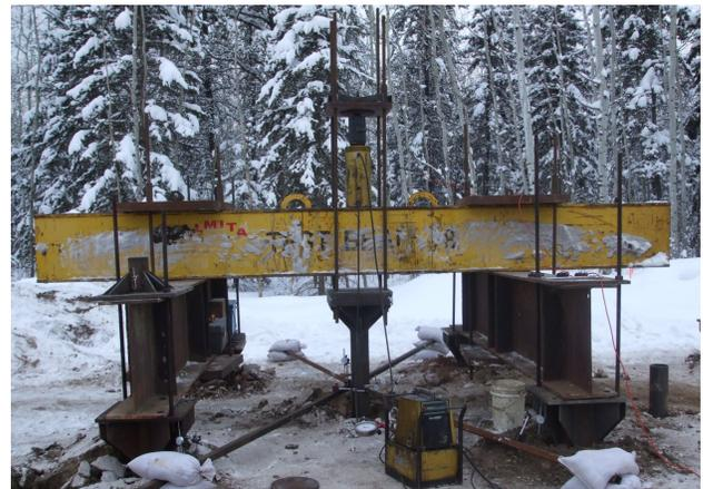
Figure 3 Test setup for uplift pile load test (Phase 2)
