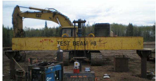
Figure 2 Test setup for uplift pile load test (Phase 1)
