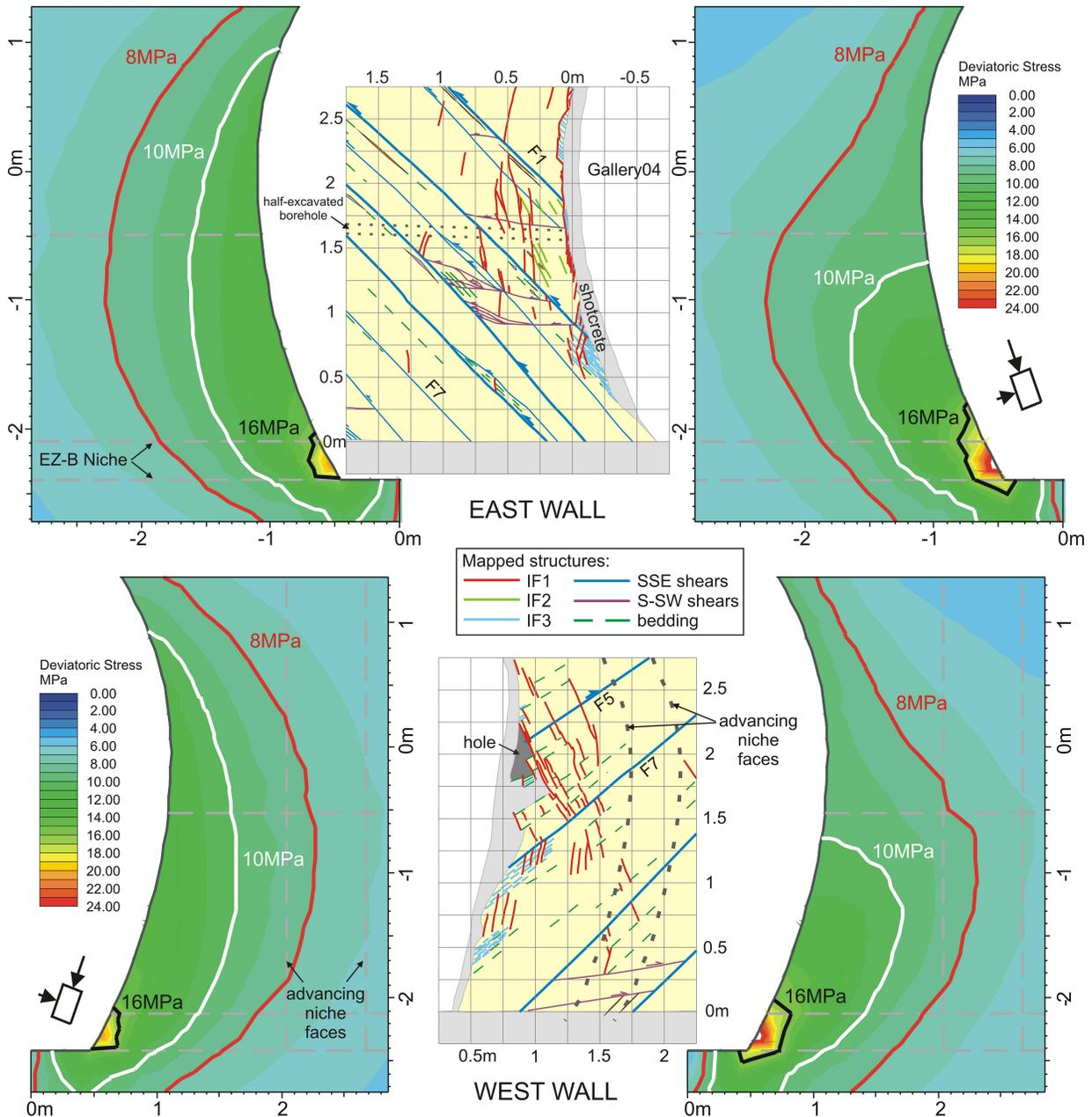
Figure 4. Deviatoric stress contours of elastic isotropy (left) compared to elastic transverse isotropy (right) without consideration of the tectonic shears. East niche entrance wall in the top and west niche entrance wall in the bottom.
