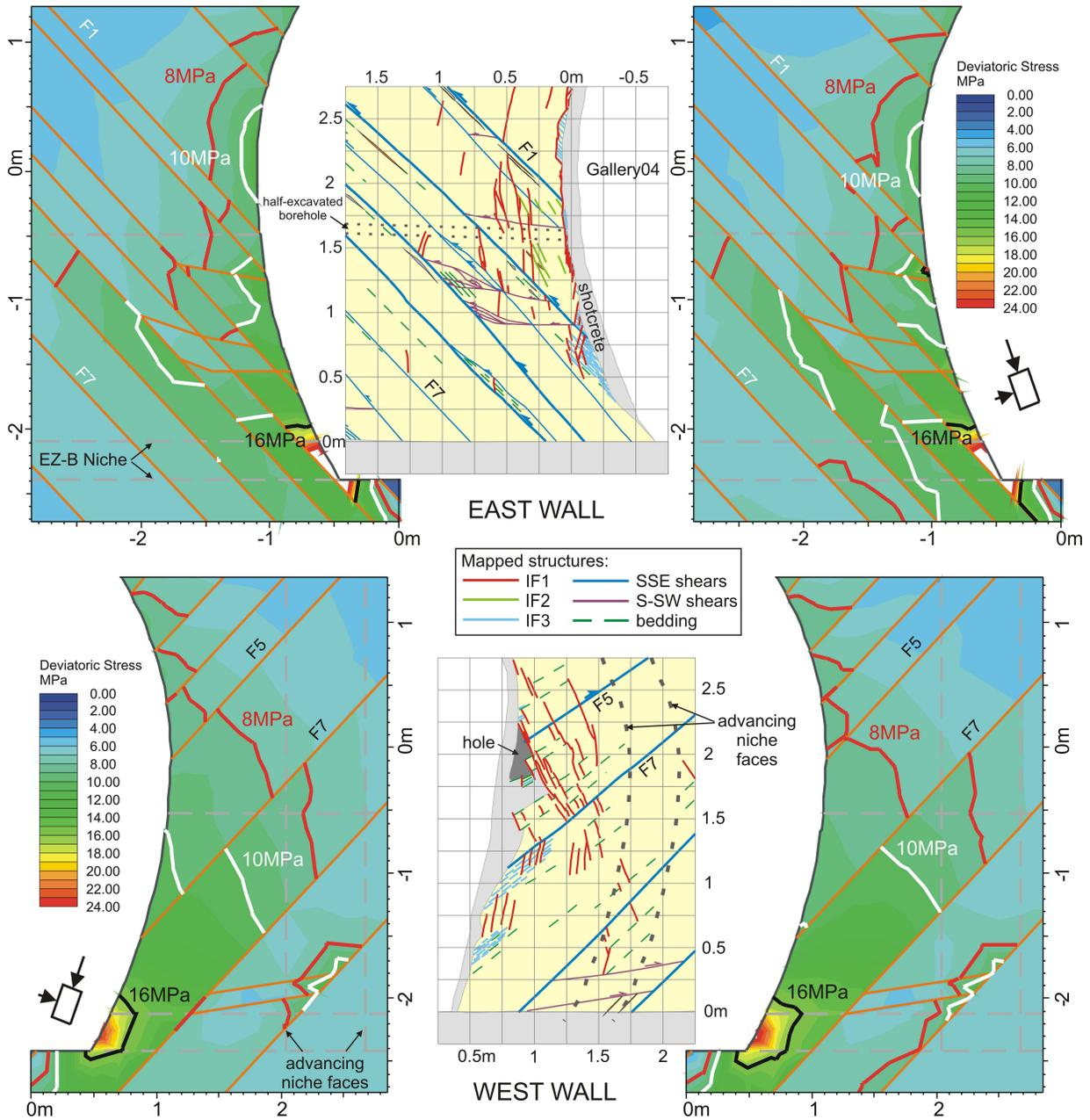
Figure 5. Deviatoric stress contours of elastic isotropy (left) compared to elastic transverse isotropy (right) with all mapped shears modelled. East niche entrance wall in the top and west niche entrance wall in the bottom.
