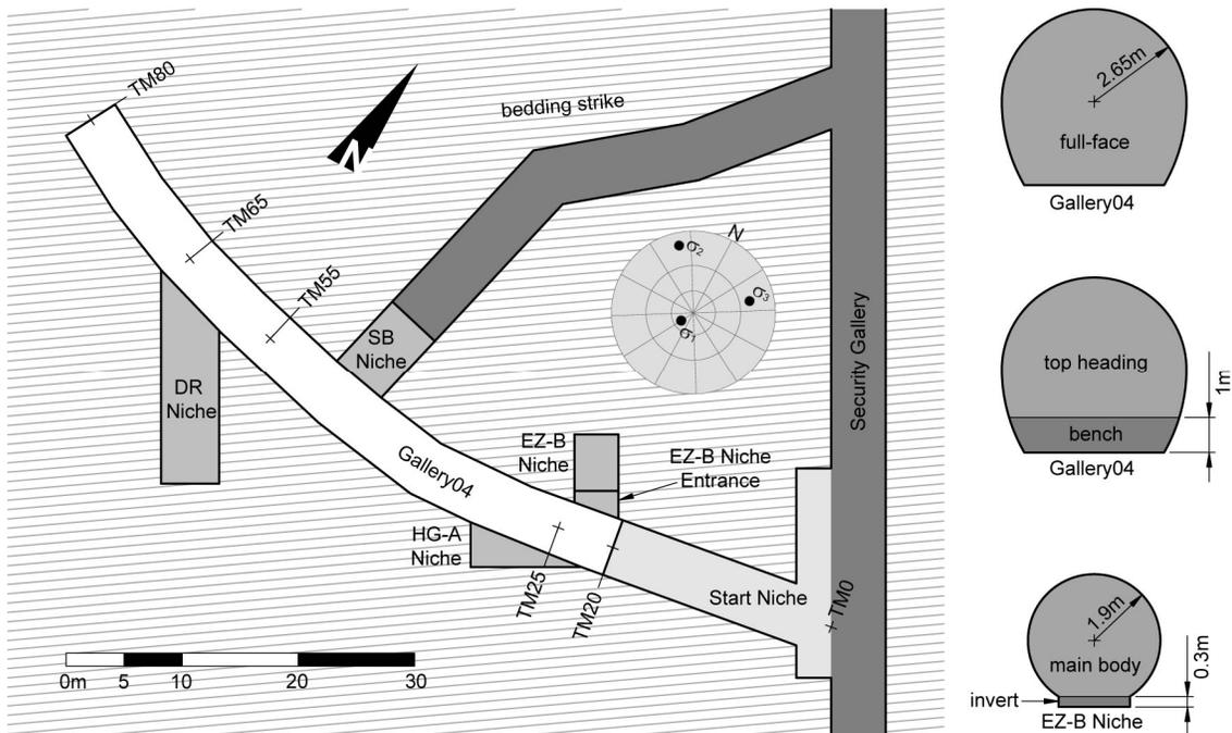
Figure 2. Layout of the Rock Laboratory around the EZ-B Niche and in situ stress field (lower hemisphere) with cross-sections of Gallery04 and the EZ-B Niche to the right.
