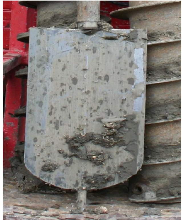
Figure 12: Specialized cutting tools for pressure cell
